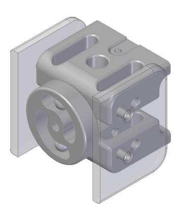
Portion of jaw mechanism (parts hidden/transparent for clarity)
