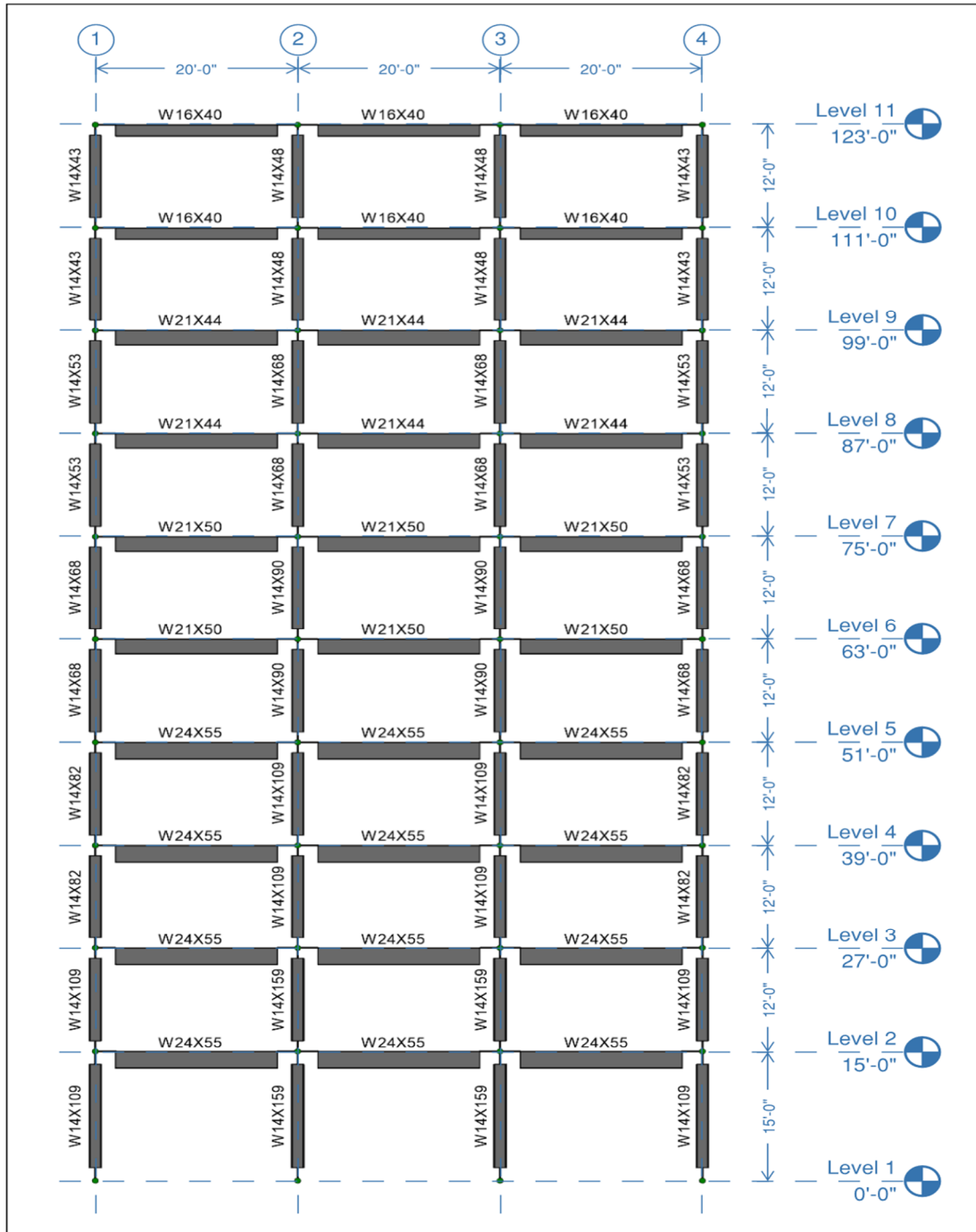
Figure 12.3 - Moment Frame Elevation with Member Sizes and Dimensions Shown
