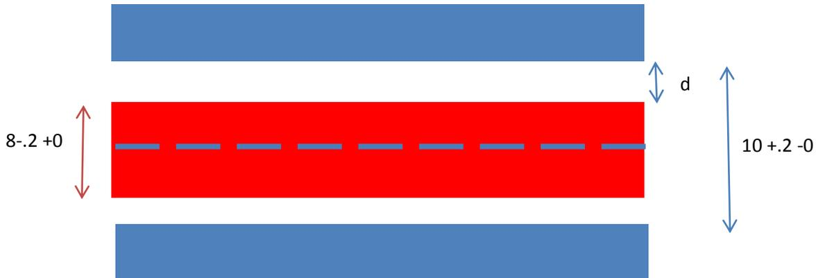
The correct result of this stackup should be that the distance can be anywhere from 0 to 2.4, depending on the diameter of each part and where the inner part is shifted with respect to the first part. The mean value for the gap should be 1.1, which is the gap if the two components are made to center tolerance and have the same center axis.
