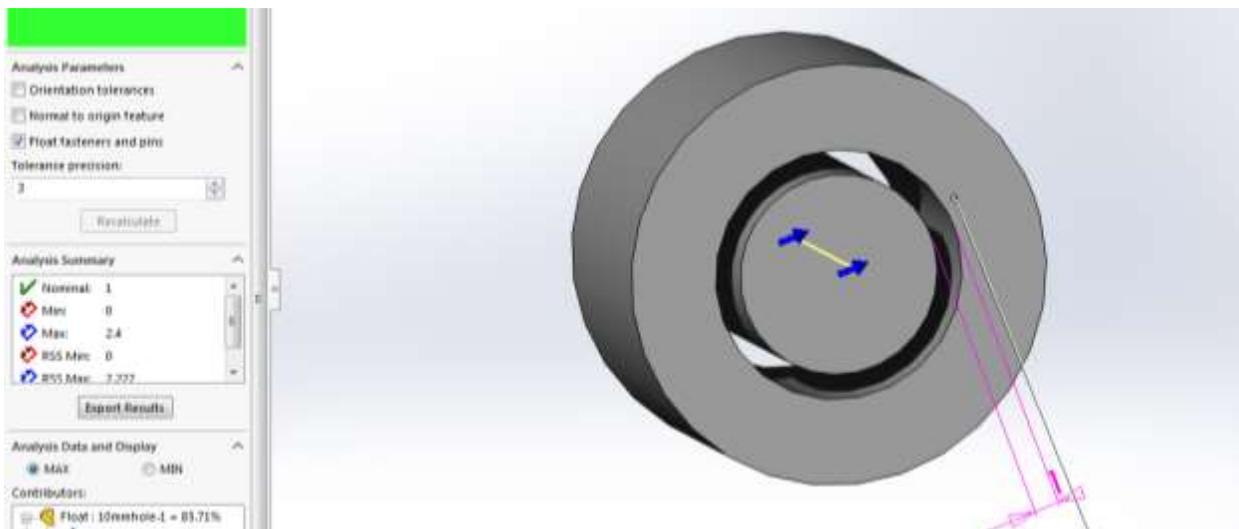
However, Sigmetrix CETOL calculates the worst case min and max gap to be  $-0.2$  to 2.4 respectively.
