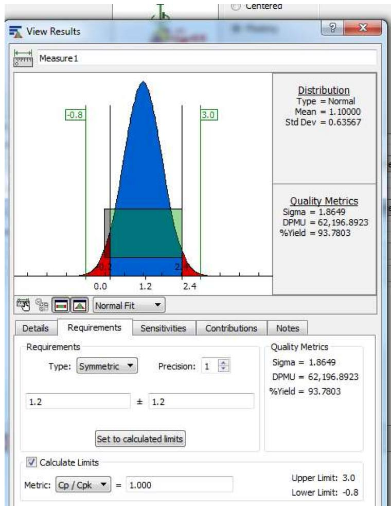
A gap of -.2 seems to indicate that interference is possible, depending on the diameters of each component. Of course, this is not possible as the 8mm shaft is always smaller than the 10mm mating diameter. I've doublechecked my CETOL setup numerous times and believe I am setting up the problem correctly. How can a commercial package like CETOL provide a wrong answer for the minimum gap. calculating possible interference is very important for the products I am working on.
