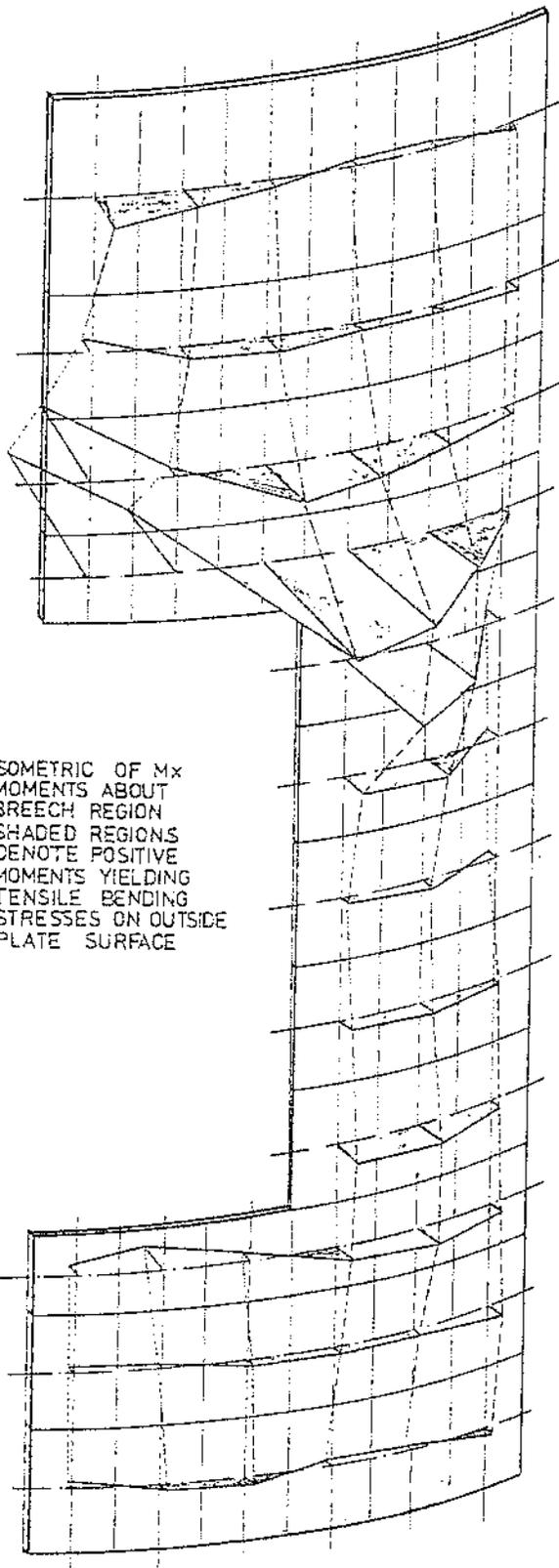
FIGURE 5.51 — Isometric plot of moment,  $M_x$  around opening.
