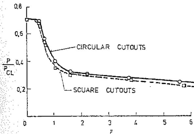
FIGURE 5.26 — The effect of circular and square cutouts on the buckling of a circular cylinder loaded by central axial compression.
