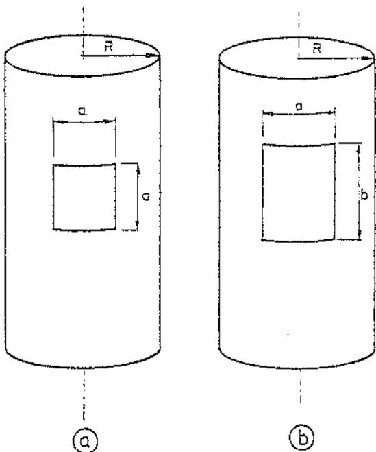
FIGURE 5.24 — Square and rectangular cuts in cylinders.
