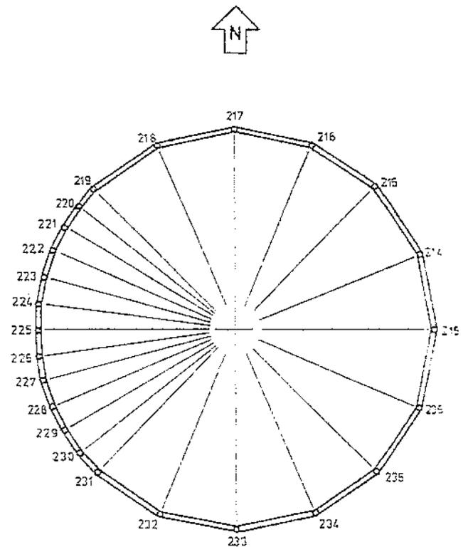
FIGURE 5.42 — Plan cross-section at El. = 50' cross-sectional radius = 170.375".
