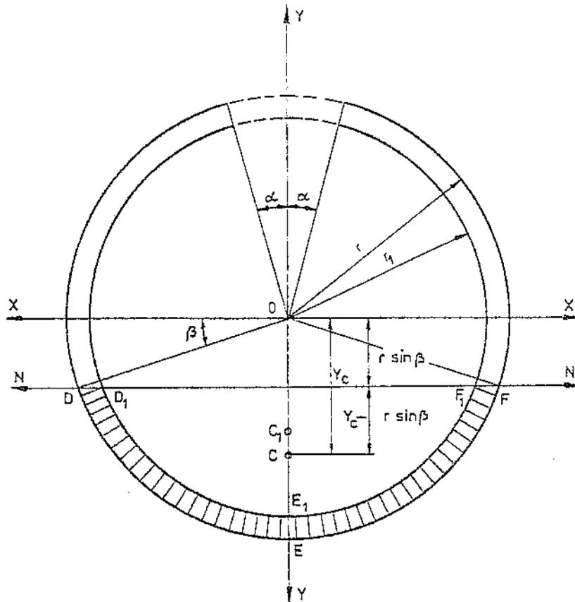
FIGURE 5.20 — Geometric data for determination of statical moment of tensile area.
