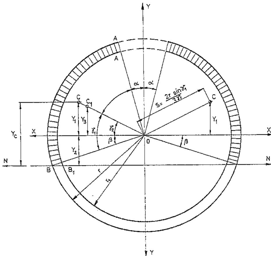
FIGURE 5.19 — Geometric data for the determination of statical moment of compressed area.
