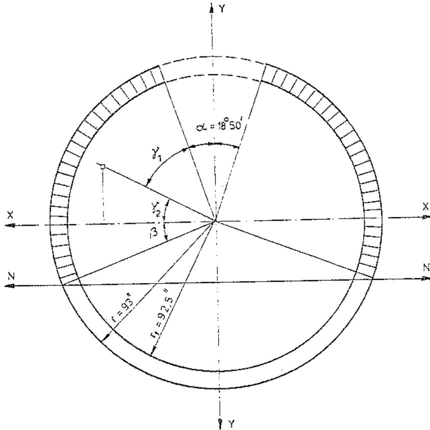
FIGURE 5.36 — Geometric data for statical moments of compressed and tensile areas.
