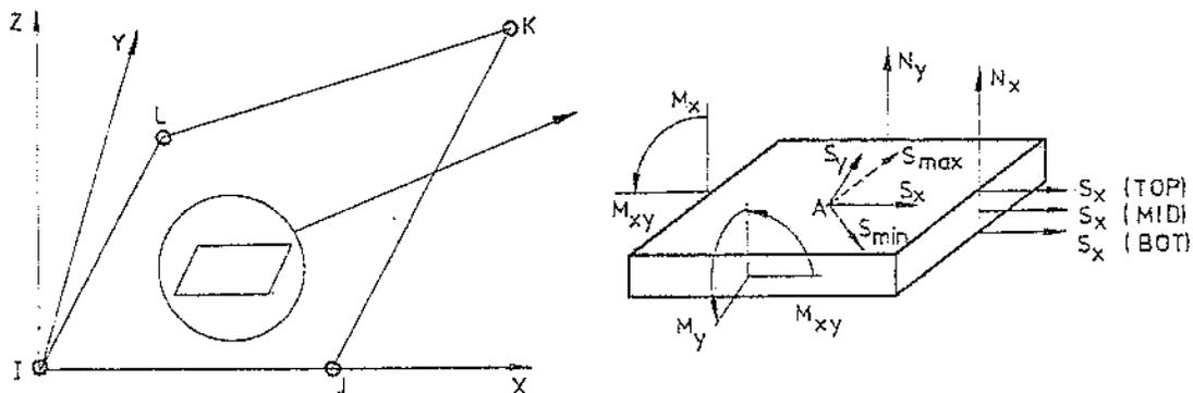
FIGURE 5.32 — Flat quadrilateral shell element output.
