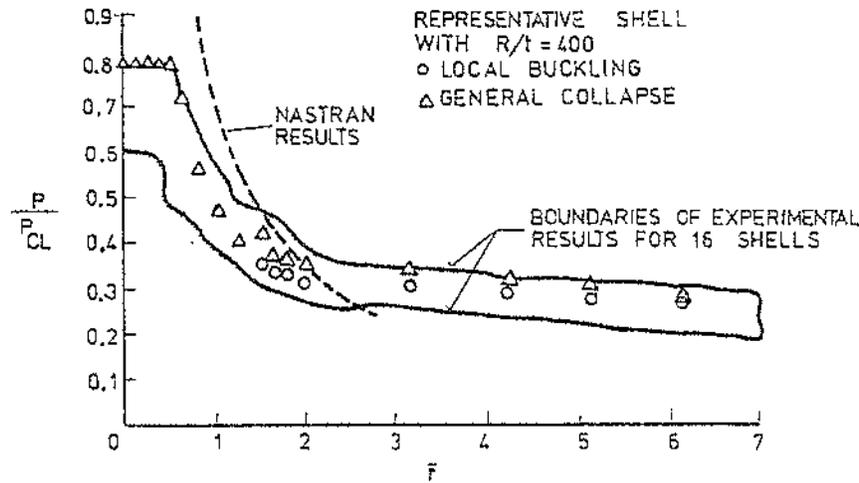
FIGURE 5.25 — The effect of circular cutouts on the buckling of circular cylinders loaded by central axial compression.
