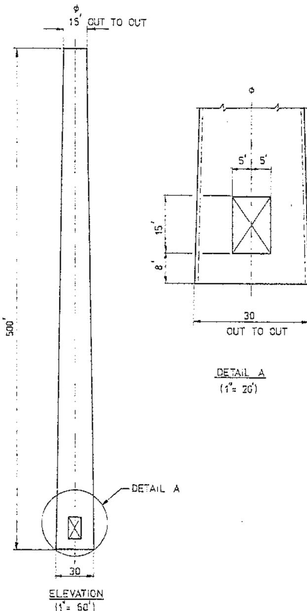
FIGURE 5.37 — Stack and breach dimensions.
