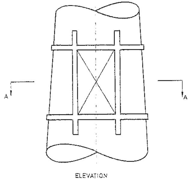
FIGURE 5.27 — Breech opening geometry.
