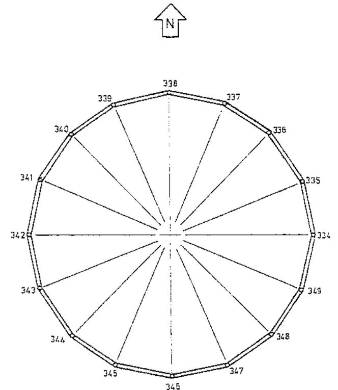
FIGURE 5.44 — Plan cross-section at El. = 180' cross-sectional radius = 157.775".
