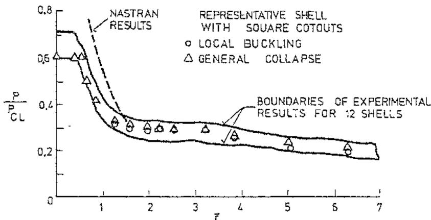
FIGURE 5-23 — The effect of square and rectangular cutouts on the buckling of circular cylinders loaded by central axial compression.
