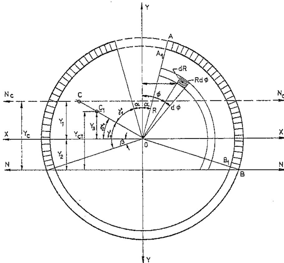
FIGURE 5.21 — Geometrical data for determination of moment of inertia of compressive area.
