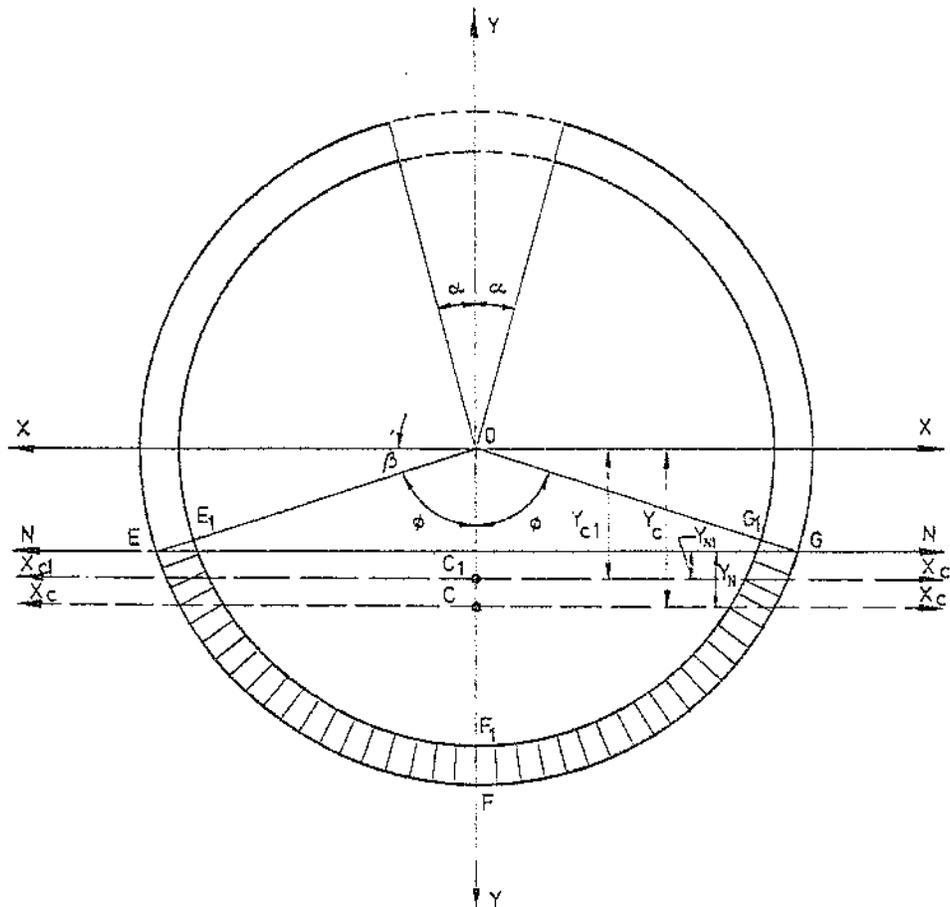
FIGURE 5.22 — Geometrical data for determination of moment of inertia of tensile area.
