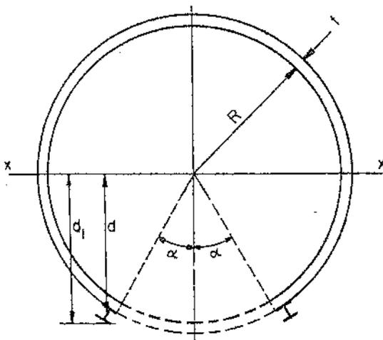
FIGURE 5.28 — Breech opening and stiffeners geometry.
