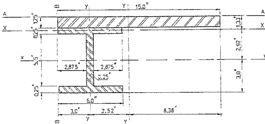
FIGURE 5-53 — Composite vertical stiffener and stack plate section.
