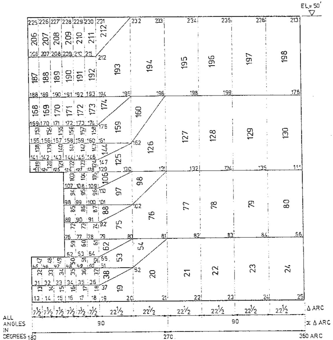
NOTE: The discretization scheme presented on Figure 5.40 is a developed view of the right half (with respect to the opening) of the truncated cone between stack elevations 0.0 and 50.0. The regular shaped elements i.e. rectangles and triangles, as shown, are in fact distorted with vertical lines slightly inclining to the left and the horizontal ones with some curvature.
