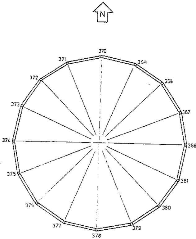
FIGURE 5.45 — Plan cross-section at El. = 160' cross-sectional radius = 150.575".
