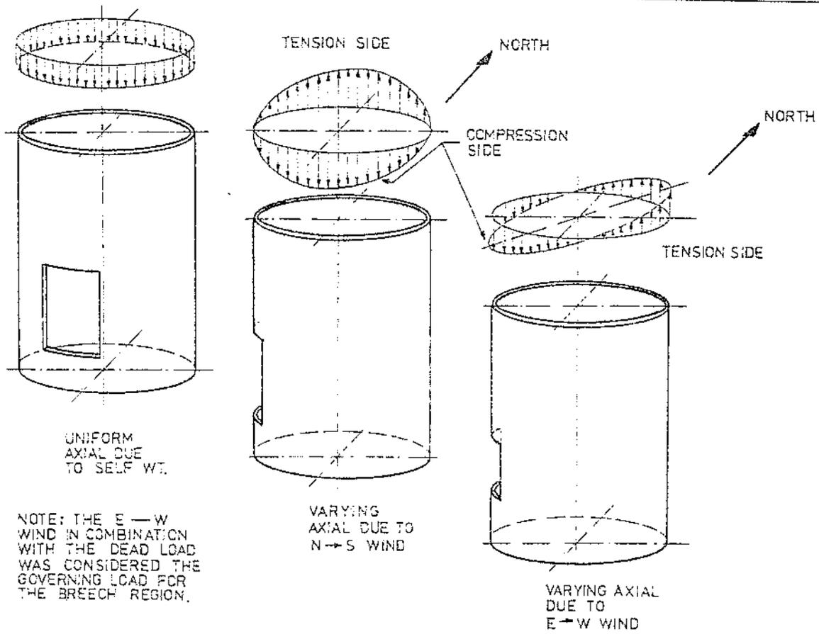
FIGURE 5.49 — Model II top edge vertical line loads due to lateral wind and self-weight dead load.
