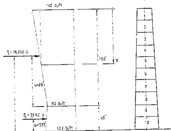
FIGURE 5.34 — Determination of bending moments in stack under wind loading.
