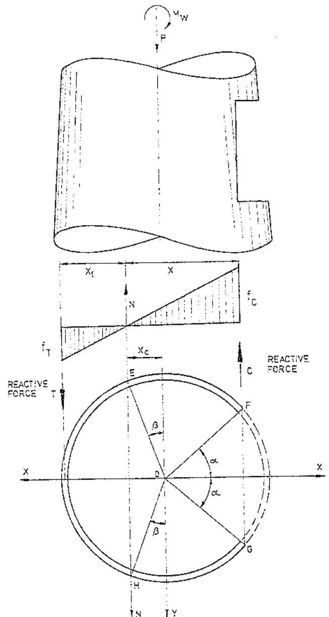
FIGURE 5.17 — Cross-section of the stack. Stress distribution diagram.
