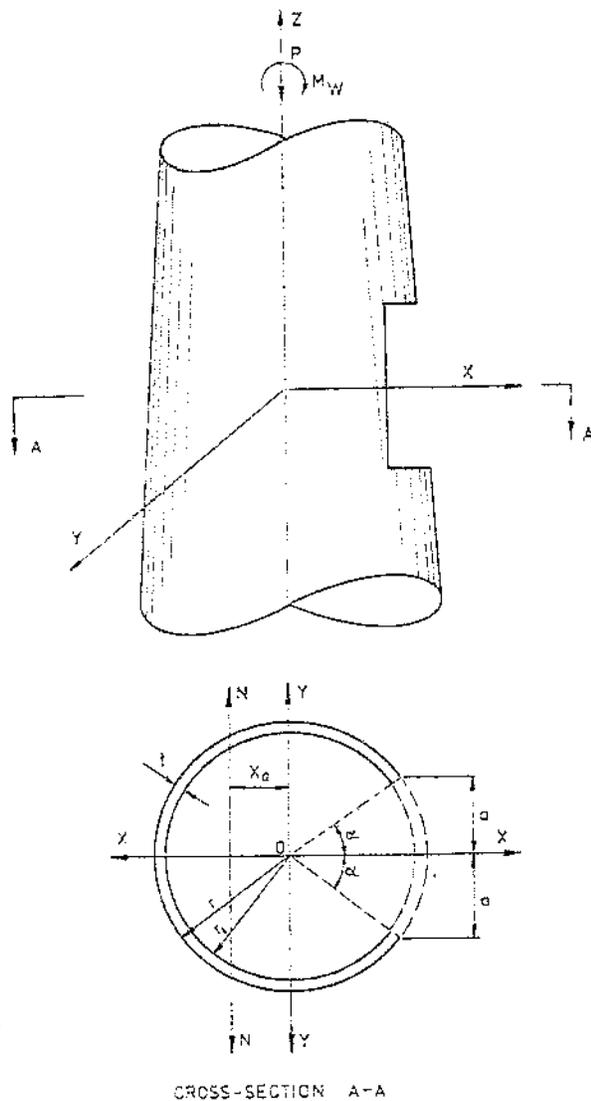
FIGURE 5.16 — Shell and hole geometry.
