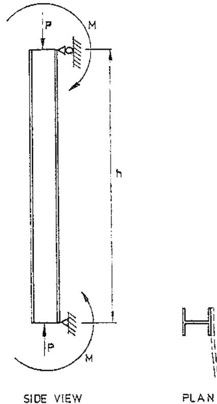
FIGURE 5.29 — Vertical stiffener as beam-column.
