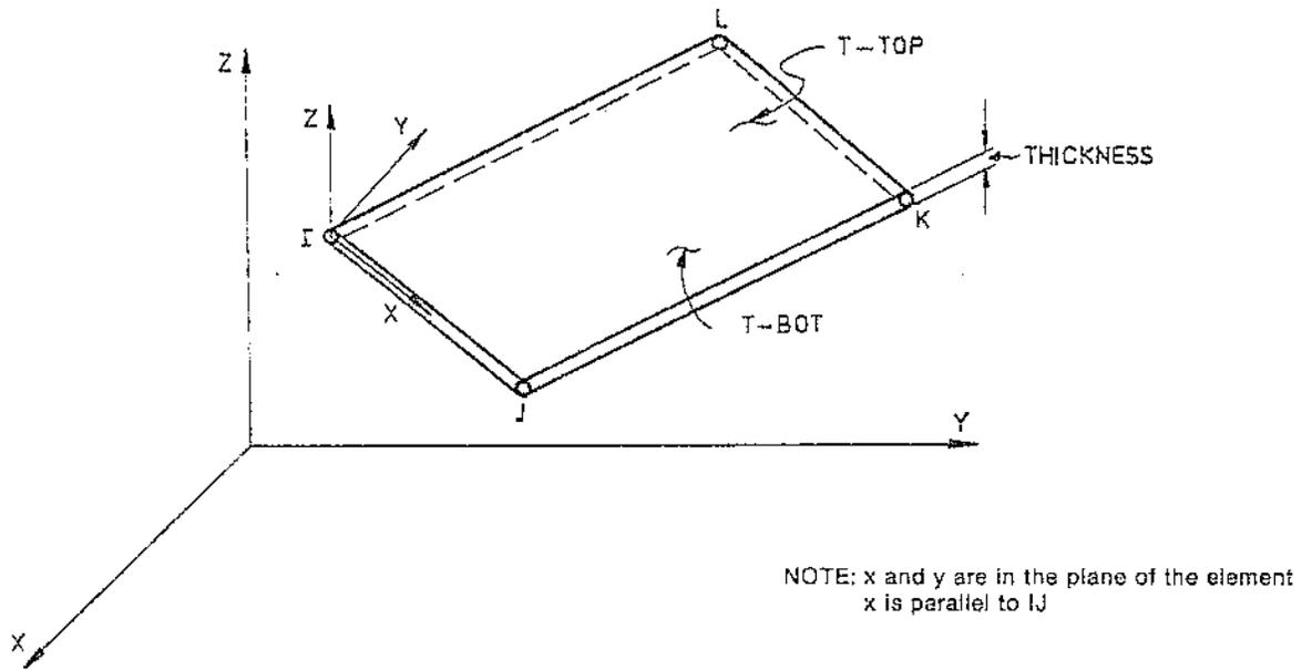
FIGURE 5.31 — Flat quadrilateral shell element.
