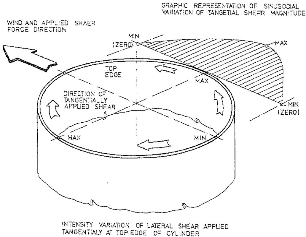
FIGURE 5.50 — Lateral shear along cylindrical plan cross-section.
