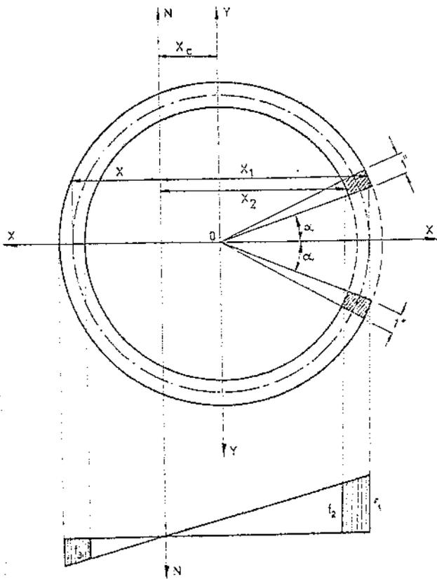
FIGURE 5.18 — Diagram of stresses in the wall of stack.
