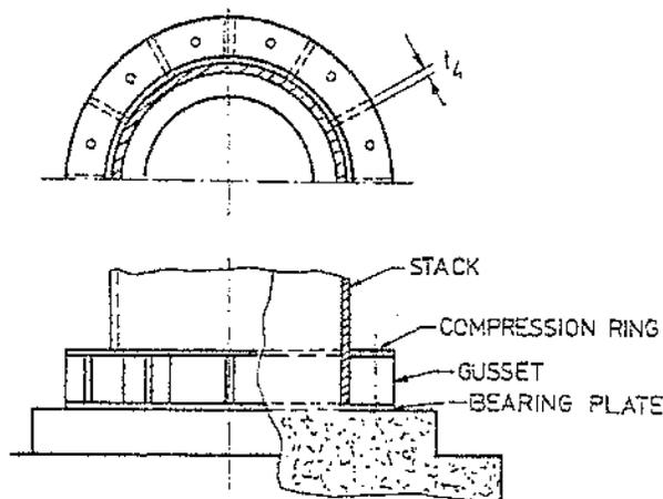
FIGURE 5.15 — Stack shell with external bolting chairs.
