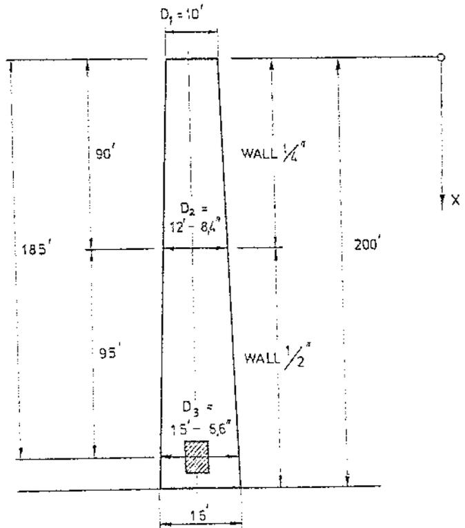
FIGURE 5.35 — Stack's wall dimensions.
