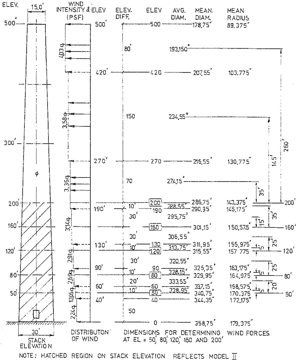
FIGURE 5.48 — Model II region and dimensions required to determine wind forces at node elevations shown.
