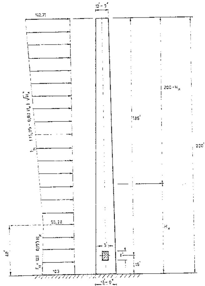
FIGURE 5.33 — Distribution of wind load acting on the stack.
