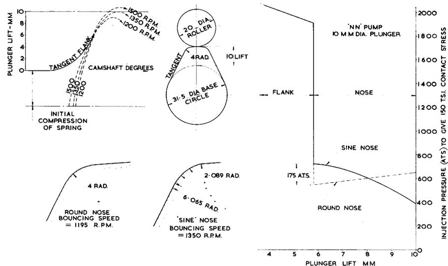
Fig. 12.—The Sine Nose Cam.
