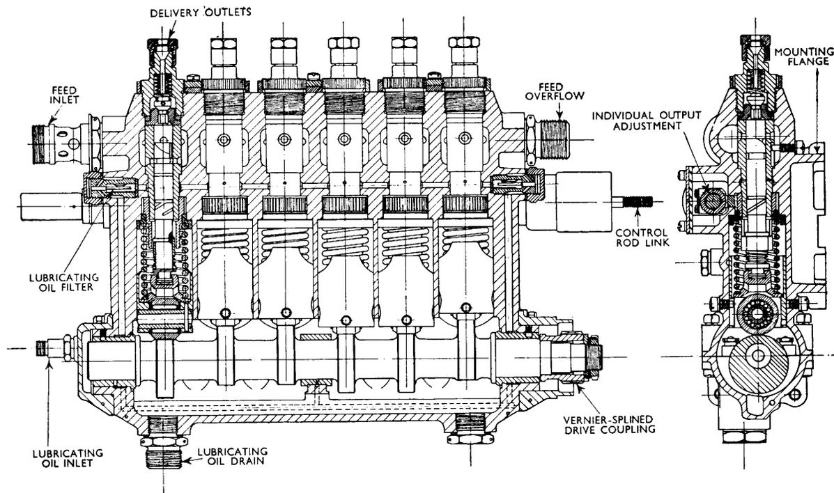
Fig. 3.—Petrol Injection Pump for Rolls-Royce "Crecy" Engine.
