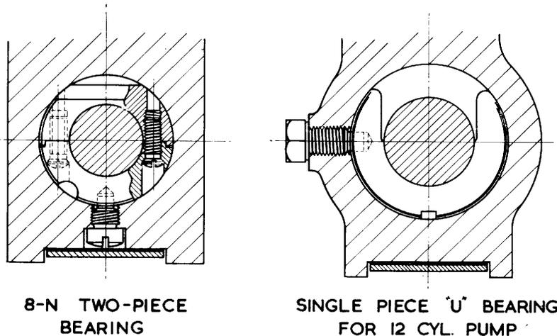
Fig. 17.—Camshaft Intermediate Bearings.
