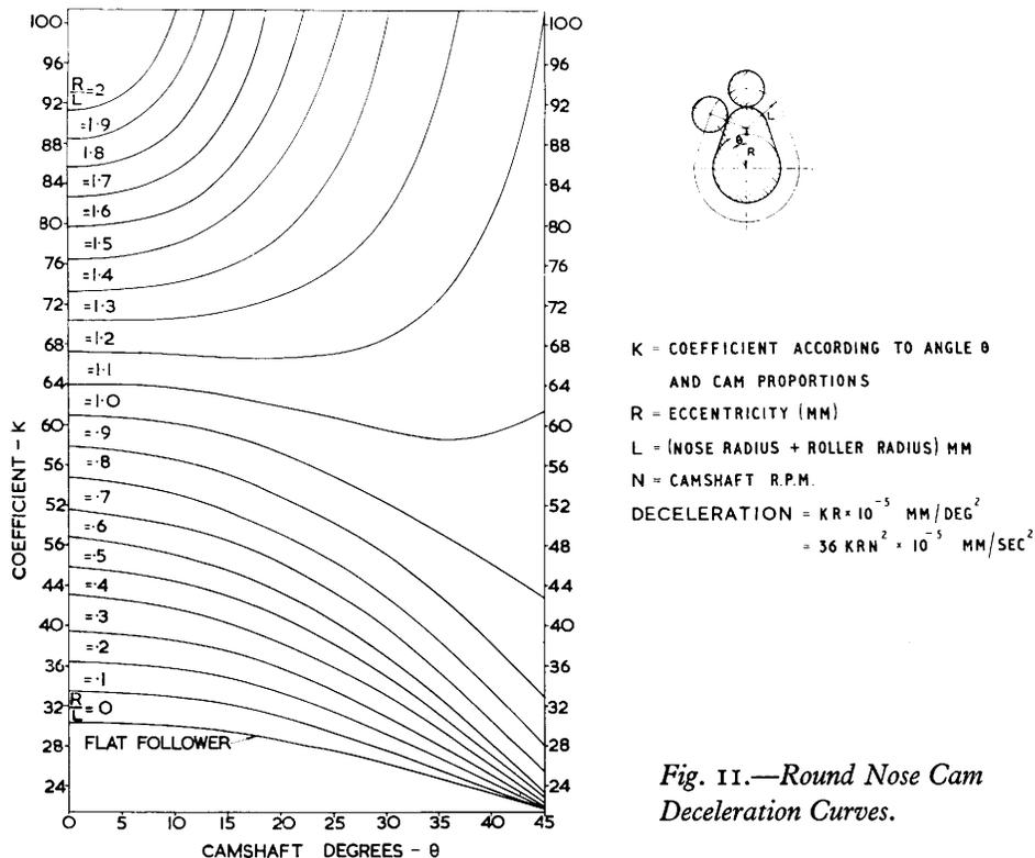
Fig. 11.—Round Nose Cam Deceleration Curves.
