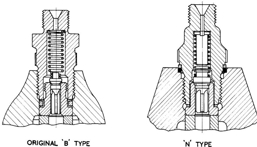
Fig. 8.—Comparison of Delivery Valve Assemblies.
