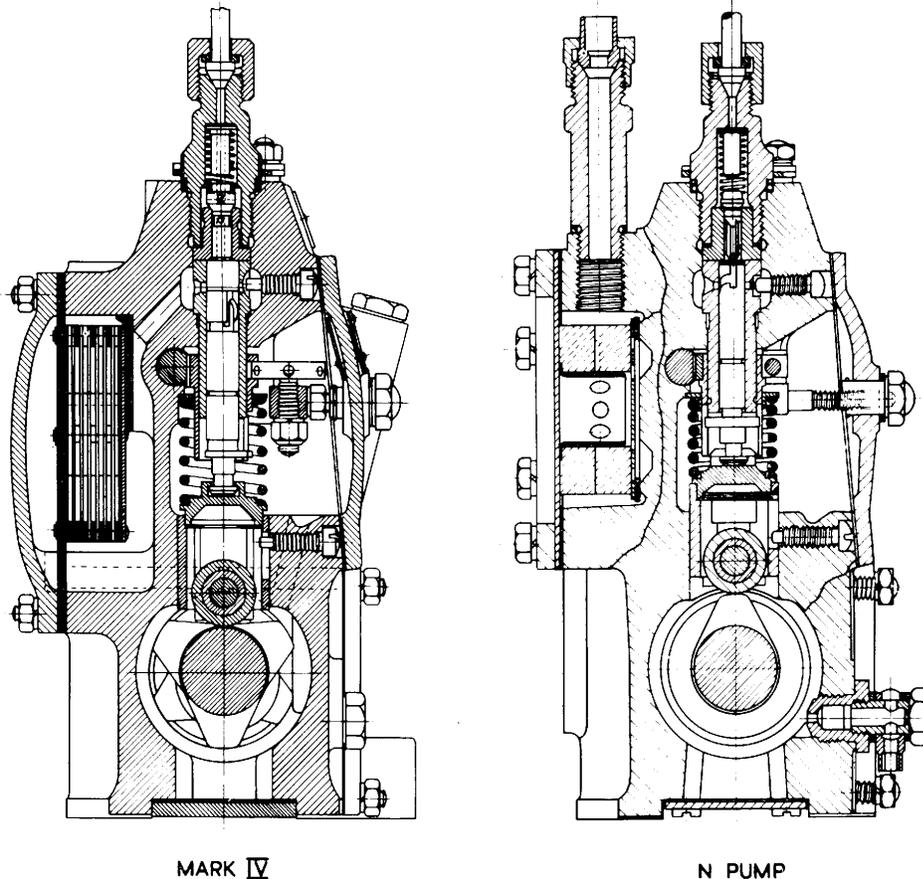
Fig. 5.—'N' Pump development—Mark IV and final production design.
