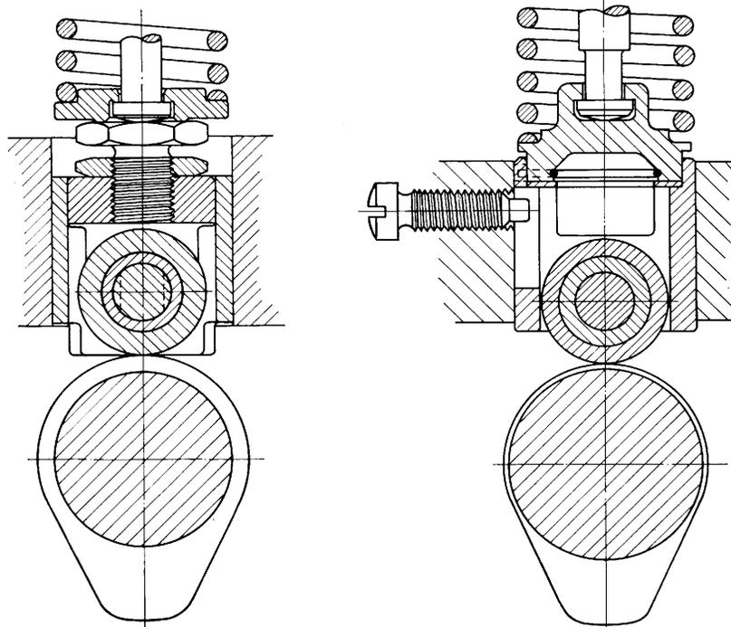
Fig. 10.—Comparison of Tappet Assemblies.
