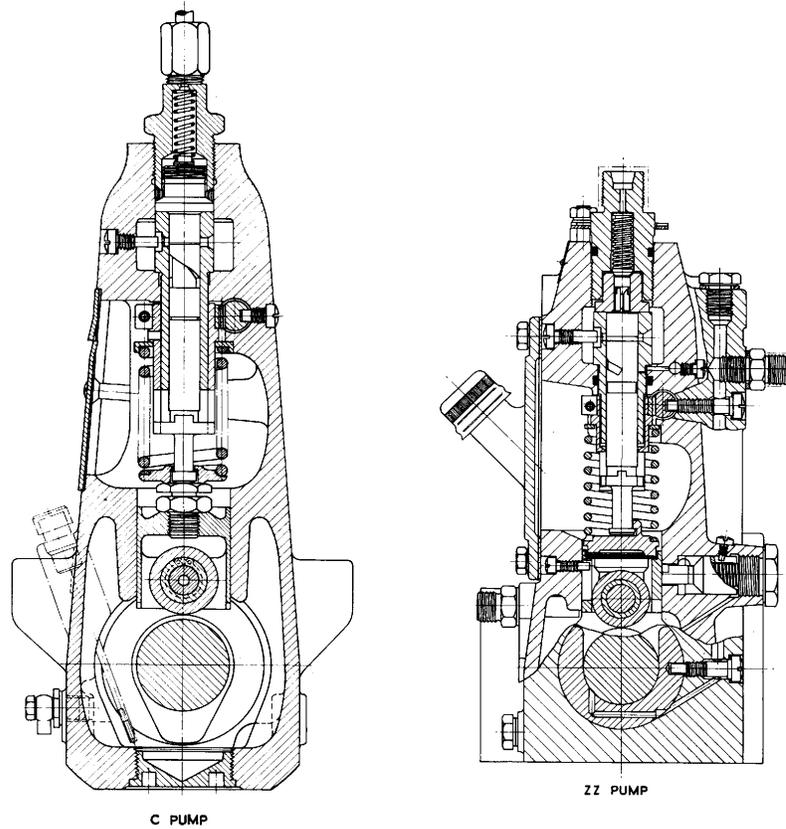
*Fig. 22.—Comparison of 'C' and 'ZZ' Pumps.*
