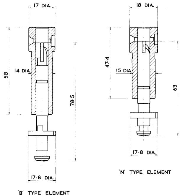
Fig. 7.—Comparison of Pumping Elements.
