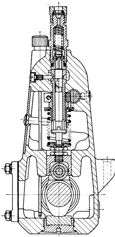
Fig. 2.—Original 'B' Type Pump.
