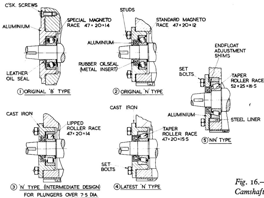
Fig. 16.—Development of Camshaft End Bearings.
