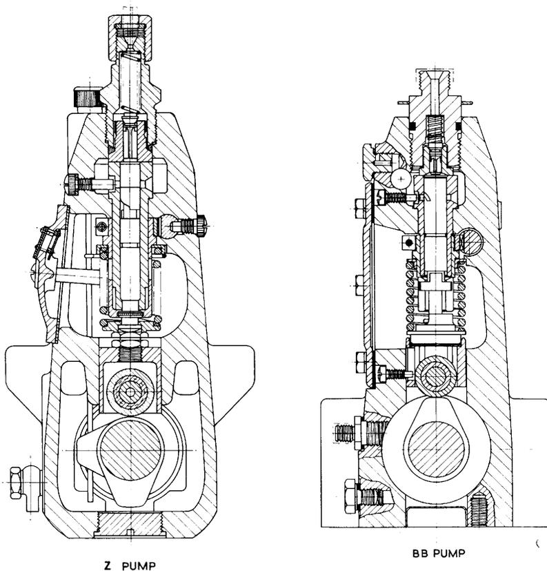
Fig. 21.—Comparison of 'Z' and 'BB' Pumps.
