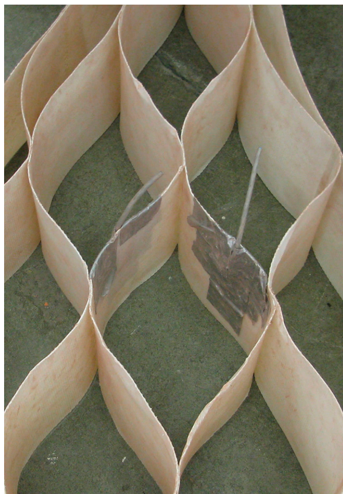
Fig. 8. Cosmetic damage to geocell consisting of only minor bending and scraping
