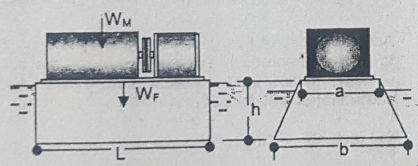
1. Knowing the bedplate dimensions of the machine, determine the upper dimensions of the foundation "a" and "L". Allow a clearance from the edge of about one foot or about 10% of the length of the bedplate.
