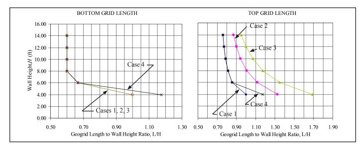
Figure 3—Flat Slope Cases, Varying  $\phi$ ,  $\gamma$  and q—Cases 1, 2, 3 and 4
