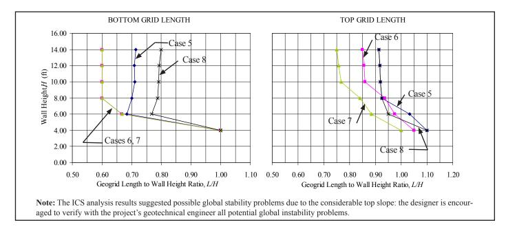
Figure 4—3:1 Top Slope Cases, Varying  $\phi$  and  $\gamma$ —Cases 5, 6, 7 and 8
