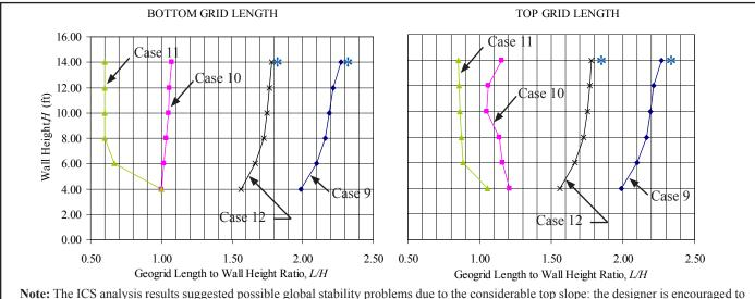
Note: The ICS analysis results suggested possible global stability problems due to the considerable top slope: the designer is encouraged verify with the project's geotechnical engineer all potential global instability problems.
