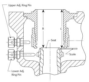
Figure 29: Guide - Bushing Seat Assembly
