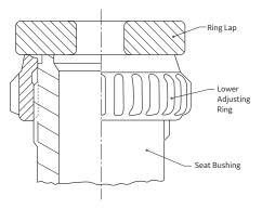
Figure 28: Bushing Seat Assembly
