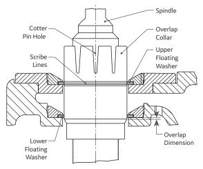
Figure 32: Collar and Spindle Assembly
