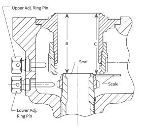
Figure 14: Guide - Bushing Seat Assembly
