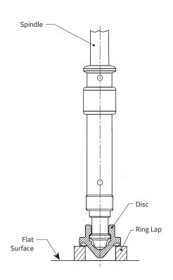
Figure 23: Disc - Spindle Bearing
