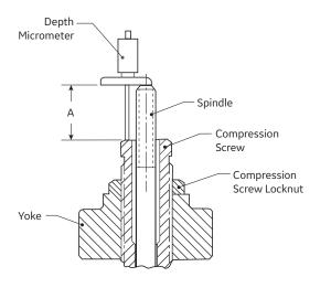
Figure 11: Yoke-Spindle Assembly
