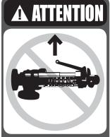
Do not lift valve horizontally, or hook to lifting lever or spring.
