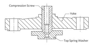
Figure 26: Compression Screw Assembly
