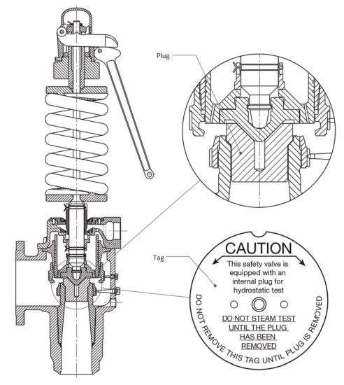
Figure 36: Hydrostatic Test Plug
