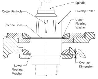
Figure 12: Collar and Spindle Assembly
