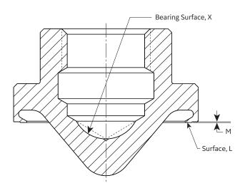
Figure 18: Thermoflex Disc
