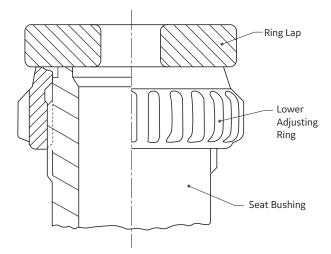
Figure 16: Bushing Seat Assembly
