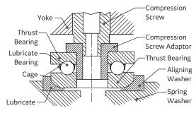
Figure 27: Thrust Bearing Assembly
