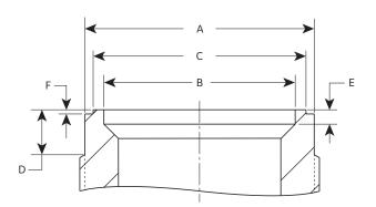
Figure 20: Seat Bushing Dimensions
