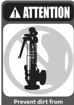
Prevent dirt from entering the outlet or inlet port.
