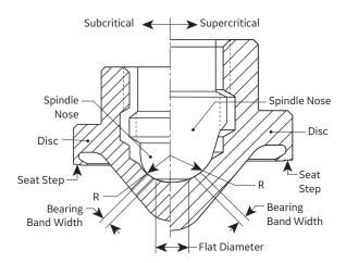
Figure 24: Disc - Spindle Assembly
