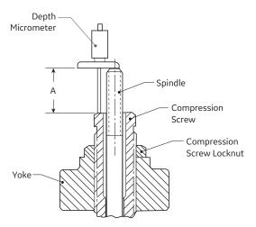
Figure 31: Yoke-Spindle Assembly
