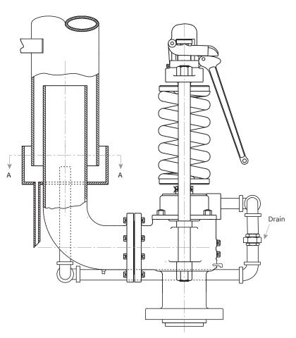
Figure 10: Recommended Installation
