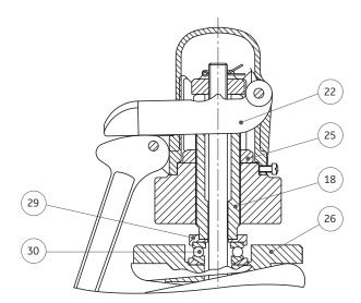
**Figure 4: Thrust Bearing**
