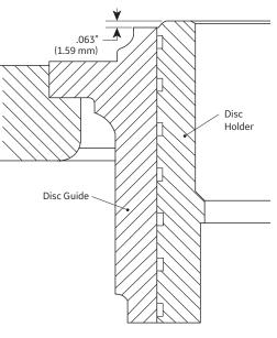
Figure 21: Guide - Disc Holder Assembly
