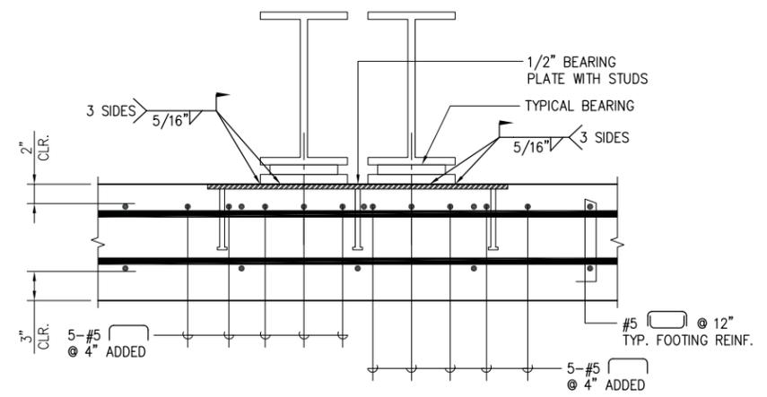
**C** BEARING PLATE SECTION AT FIXED END
