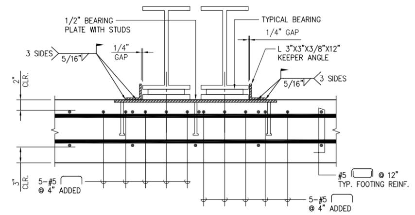
**D** BEARING PLATE SECTION AT EXPANSION END
