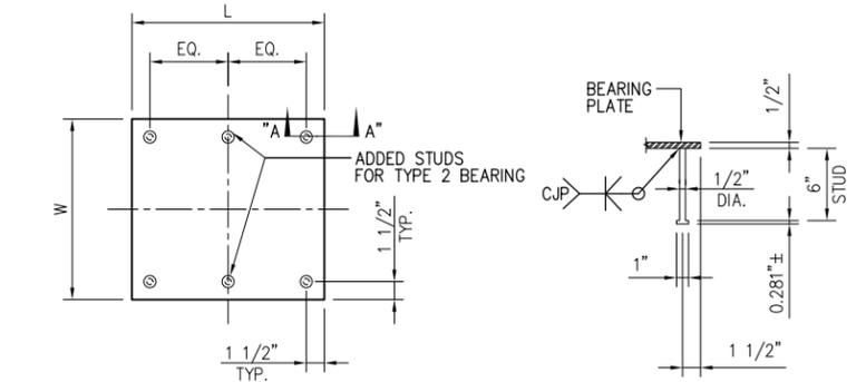
**1** BEARING PLATE WITH STUDS DETAIL
