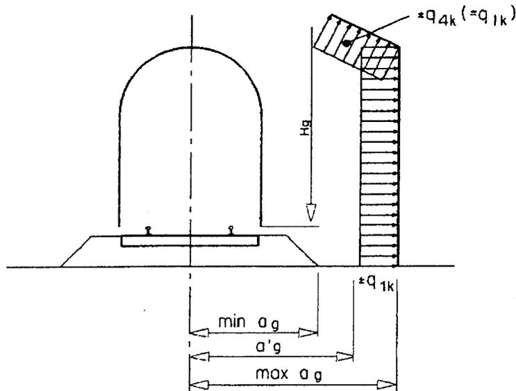
Because of the obstruction due to the second surface, the outflow of air is prevented so that the substitution loads are greater in this case than with surfaces that are simply vertical or horizontal.
