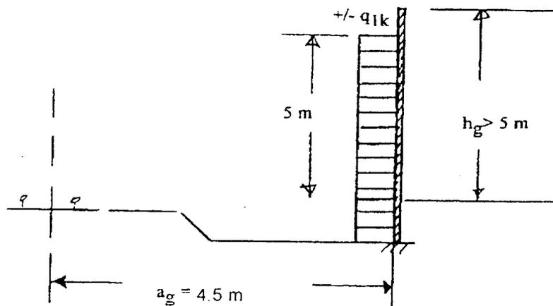
Loads  $q_{1k}$  due to the pressure-suction wave caused by the passing of a train shall be applied over the whole height of the screen, but not beyond a value 5 m above the upper level of the rail. In the direction of travel, the loads are applied over a length of 5 m with  $+ q_{1k}$  and then on 5 m with  $- q_{1k}$ .
