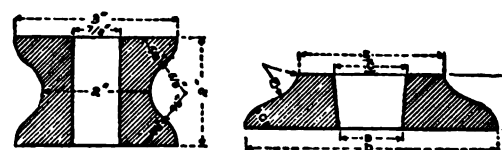
FIG. 2.—DETAILS OF SEPARATOR AND CAST WASHERS
