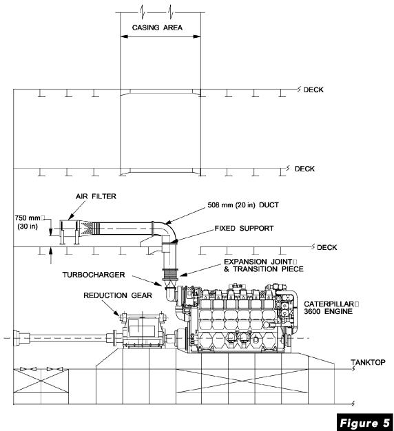
Remote Mounted Air Cleaner with Engine Room Air Intake
