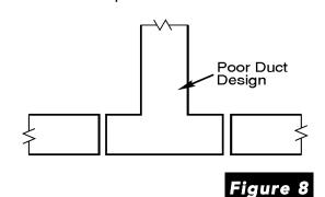
The transitions used to combine multiple ducts must also follow typical
