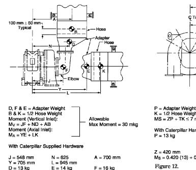
Maximum Loads for Turbocharger Intake
