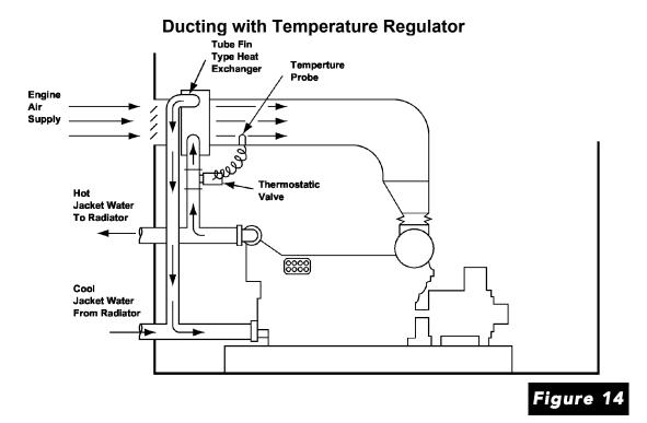
If one intake system is used to supply temperature controlled air to multiple engines, provisions must be made to ensure that heated water is sent to the heat exchanger when engines are running. If engine jacket water is used, the engine that the water is taken from must be running when any of the other engines are operating.
