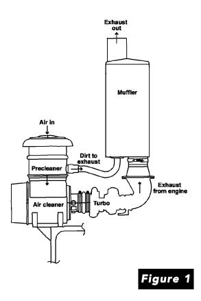
©2015 Caterpillar All rights reserved. The air comes into the precleaner where the dirt and chaff is removed from the air. With a slight vacuum, the dirt is sucked directly through the muffler into the exhaust flow and does no harm to the engine. Refer to **Figure 1**.
