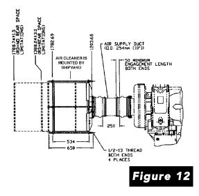
The filter/silencer provides good air filtration, but it should only be used in a clean engine room environment (filtered air). The customer is responsible for ensuring the engine room air is suitably filtered.
