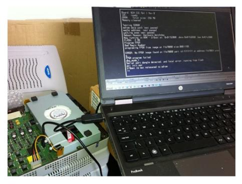
The serial port connector on a BCM 50b is located below the BRI module and you will probably need to remove the board after powering off the BCM first to insert the serial cable and then replace the module, before powering it up again as shown below with the BRI module attached. Be aware that the **bridging pins are on the right** towards the hard disk power connector.
