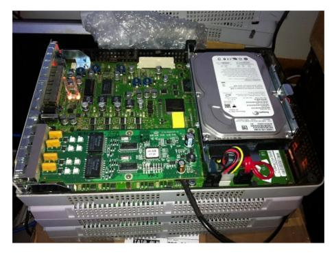
A close up of the serial cable and coloured wires is shown here attached onto a standard BCM 50. Please be aware that only three wires are needed and the Red 3.3 volts lead isn't used!. Also a green IDE jumper was used to bridge the pins needed for the u-boot console to work.
