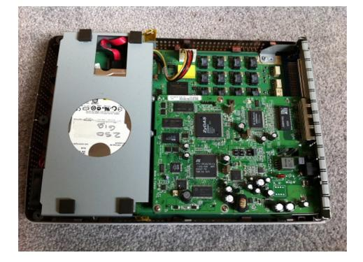
An example of a BCM 50a is shown below with the ADSL 1 card plugged in at the bottom
