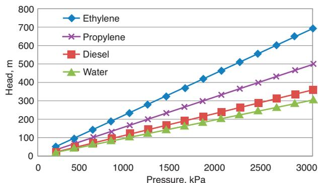
▲ Figure 3. Head required to produce similar pressures is higher for lower density fluids.
