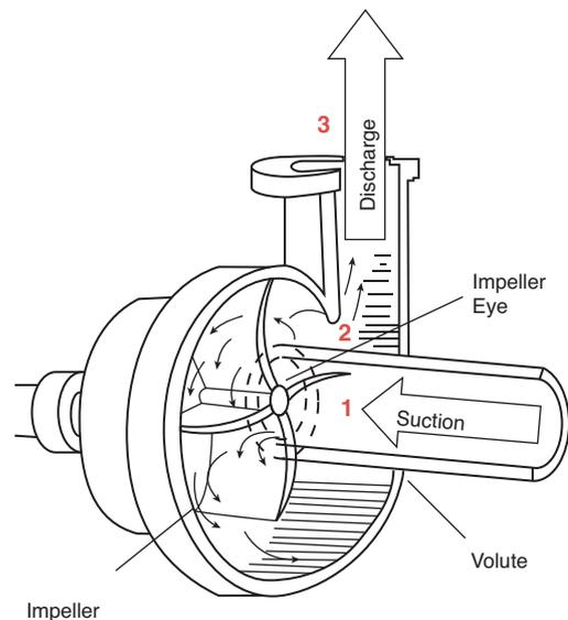
Note that the pumps illustrated in this article have open-vane impellers, which are not allowed by API 610. They are used here for illustrative purposes.
