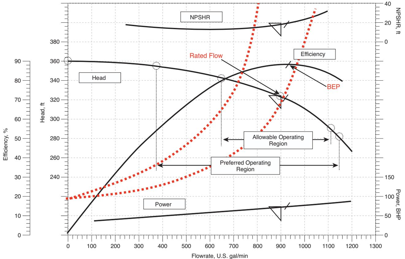
▲ **Figure 1.** The characteristics of a centrifugal pump are described by the pump performance curves. Source: (1)
