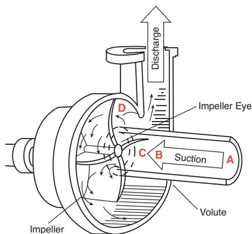
► **Figure 5.** Static pressure losses occur as the fluid travels into the pump suction and moves in and out of the impeller.
