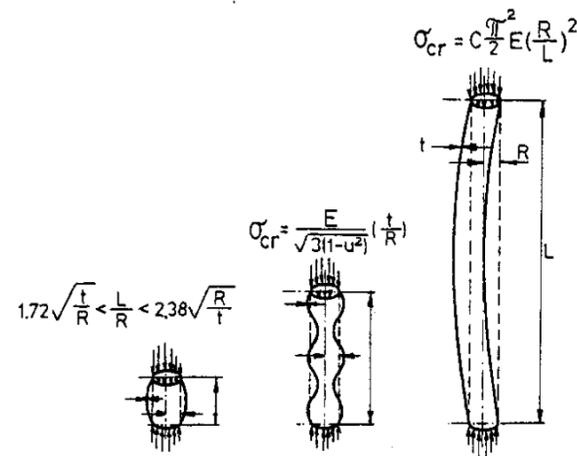
FIGURE 2.2 — Cylindrical shell subjected to axial compression.
