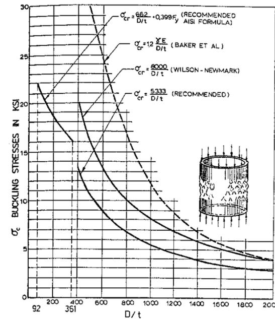
FIGURE 2.6 — The recommended allowable buckling stresses.
