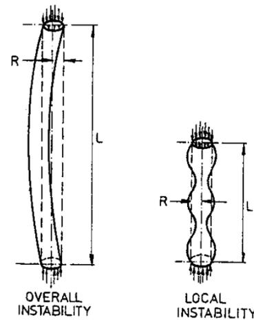
FIGURE 2.1 — Overall and local buckling.
