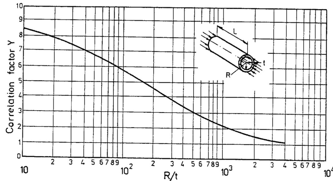
FIGURE 2.5 — Correlation factors for unstiffened circular cylinders subjected to axial compression.
