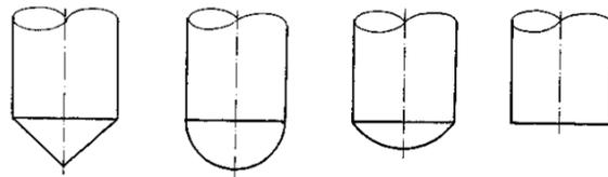
FIGURE 1.1 — Types of head-cylinder structures.
