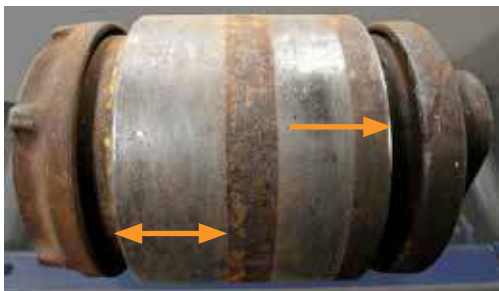
Excessive wear bands
