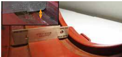
Arrows indicate an acceptable space between the toe of the gage and the machined relief of the adapter.
