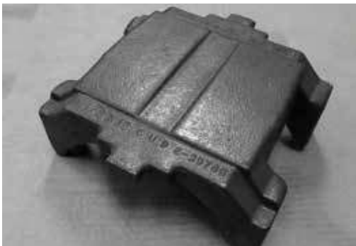
Standard freight car narrow adapter
