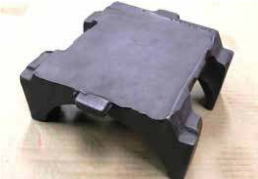
Adapter with excessive wear
