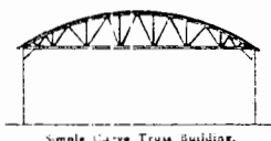
Simple Curve Truss Building.
