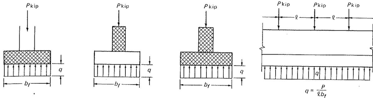
Fig. 5-9 Transforming concentrated loads into equal bearing pressures.
