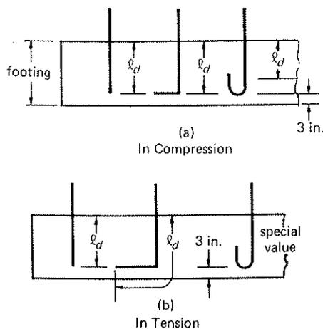
Fig. 5-25 Development (anchorage) of column bars or dowels. (a) In compression; and (b) in tension.
