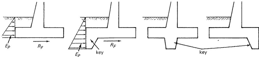
Fig. 5-41 Lateral resistance at base for retaining walls.
