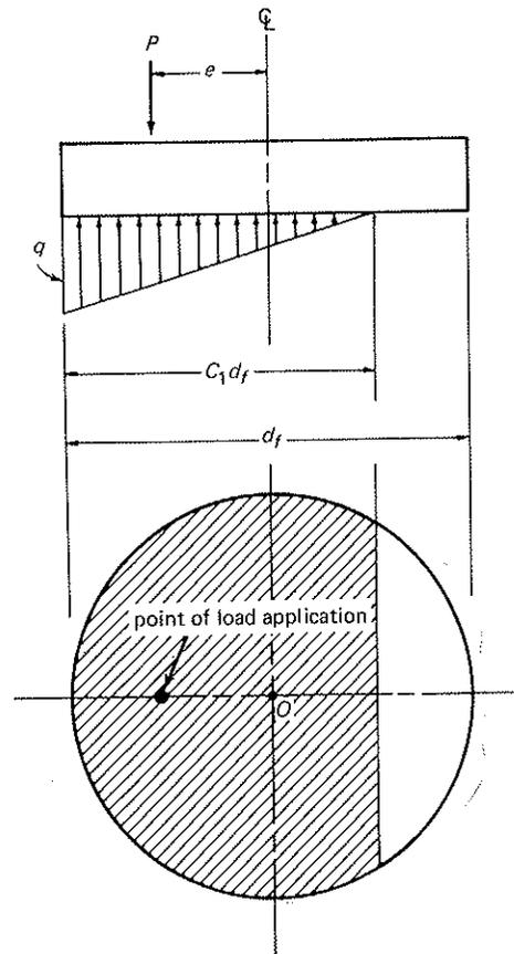
Fig. 5-14 Bearing pressure under circular and polygonal bases. Notation same as in Fig. 5-12 except for  $A_F = d_f^2 \pi/4$ .
