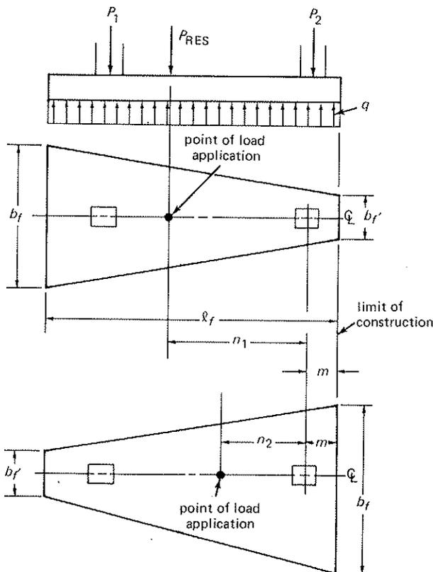
Fig. 5-18 Trapezoidal footing. \*For non-uniform bearing pressure under eccentric loadings see: A. Zweig, "Eccentrically loaded trapezoidal or round footings," *Proceedings ASCE*, ST-1, 161-168, Feb. 1966.
