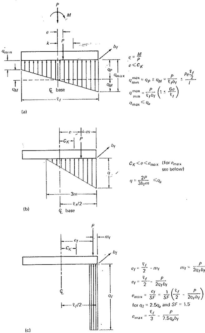
Fig. 5-5 Bearing pressure distribution under eccentric loading.
