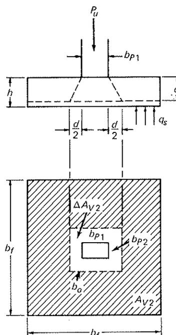
Fig. 5-29 Two-way shear action.
