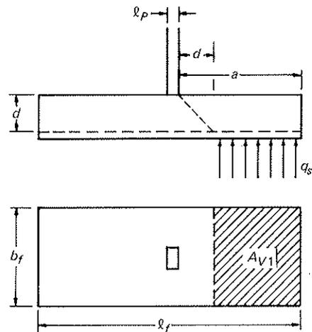
Fig. 5-33 One-way shear in oblong footings.
