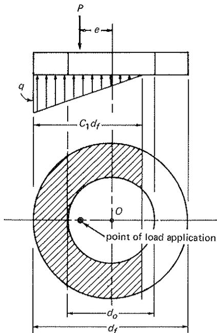
Fig. 5-15 Bearing pressure under ring-shaped bases. Notation same as in Fig. 5-12 except for  $A_F = (d_f^2 - d_o^2) \pi/4$ .
