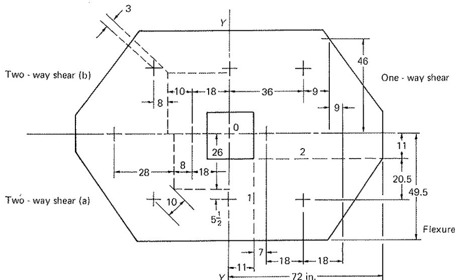
Fig. 5-38 Stress evaluation in pile caps.
