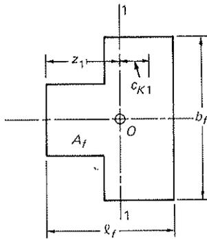
Fig. 5-4 Kern distance. (a)  $c_{K1} = I_{F1} / A_{F1} z_1$ ; (b)  $I_{F1}$  = moment of inertia of footing base about neutral axis  $I-I$ ; (c)  $z_1$  = distance of extreme fiber at opposite side of desired kern distance; (d) for strips,  $c_K = l_f/6$ .
