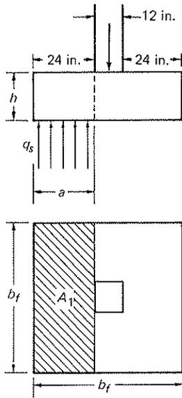
Fig. 5-35 Flexural design of structural plain concrete footings.
