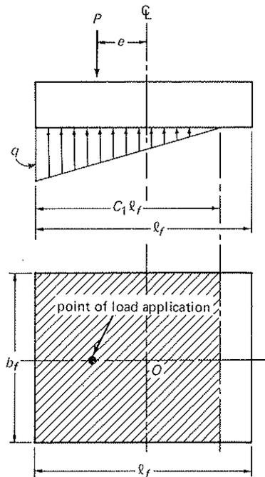
Fig. 5-12 Bearing pressure under square and oblong bases. Notation used includes:  $A_F = l_f b_f$ ;  $q_p = P/A_F$ ;  $e = M/P$ ;  $q = C_2 q_p$ ; and  $q_p$  = bearing pressure under concentric loading.
