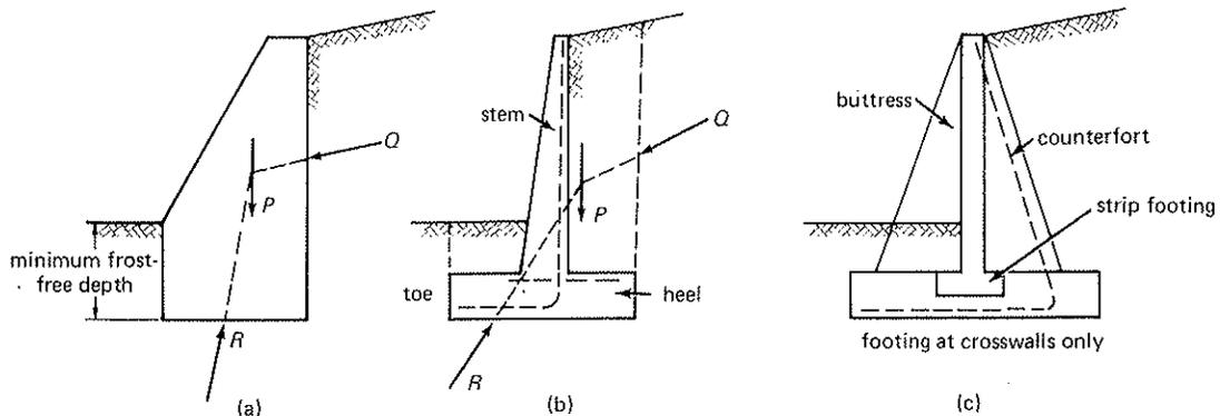
Fig. 5-39 Types of retaining walls.
