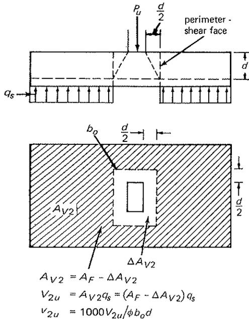
Fig. 5-23 Two-way (perimeter) shear action.
