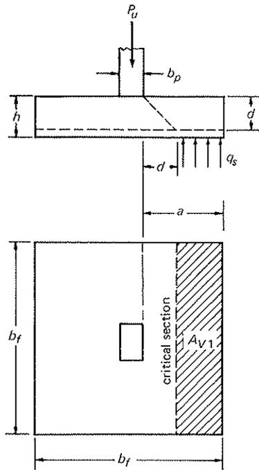
Fig. 5-30 One-way shear investigation.
