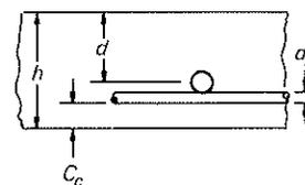
Fig. 5-32 Effective depth of spread footings.
