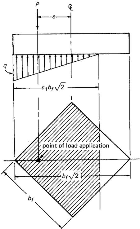
Fig. 5-13 Bearing pressure under square bases (about diagonal axis). Notation same as in Fig. 5-12 except for  $A_F = b_f^2$ .
