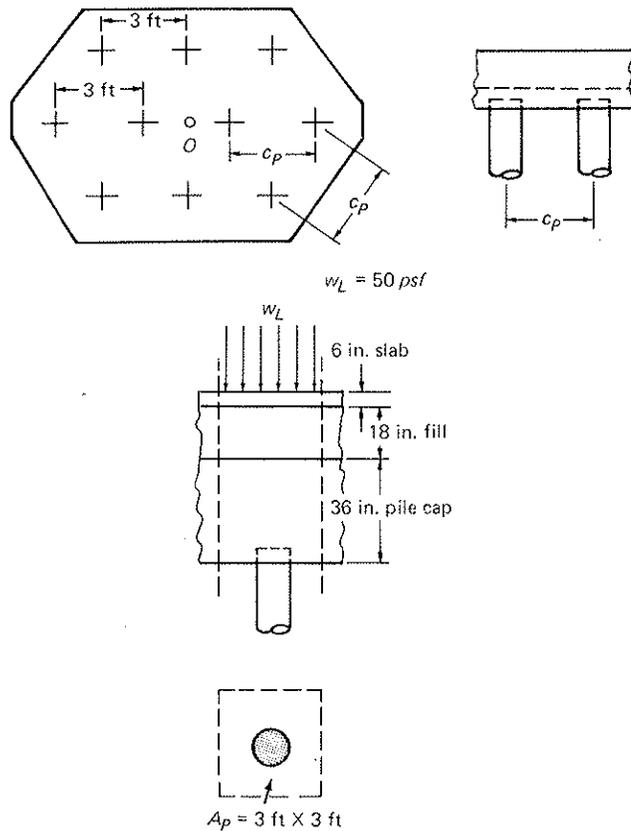
Fig. 5-37 Pile cap. Conventional pile arrangement in ten-pile cap.
