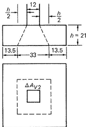
Fig. 5-36 Two-way shear in structural plain concrete footings.
