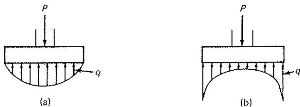
Fig. 5-1 Bearing pressure distribution for a stiff footing with frictionless base on ideal soil. (a) On cohesionless soil (sand); and (b) on cohesive soil (clay).
