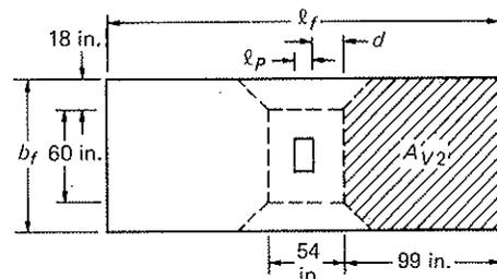
Fig. 5-34 Two-way shear in oblong footings.
