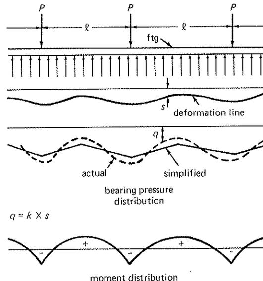
Fig. 5-6 General conditions for a beam on an elastic foundation.
