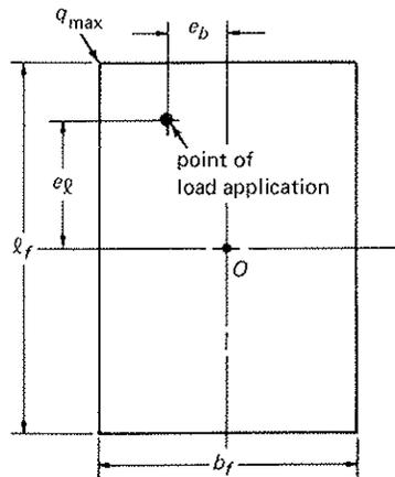
Fig. 5-16 Maximum corner pressure for biaxial eccentricities. Notation same as Fig. 5-12 except for  $q_{max} = C_3 q_p$ .
