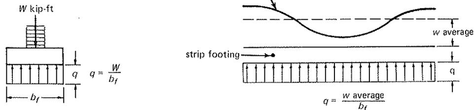
Fig. 5-8 Equalizing strip loadings of variable intensity.
