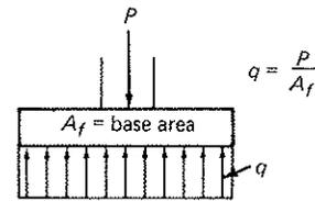
Fig. 5-3 Simplified bearing pressure distribution (commonly used).
