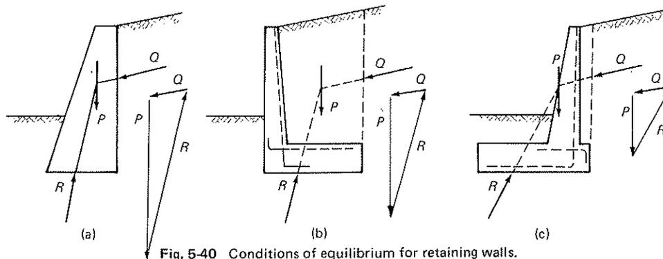
Fig. 5-40 Conditions of equilibrium for retaining walls.
