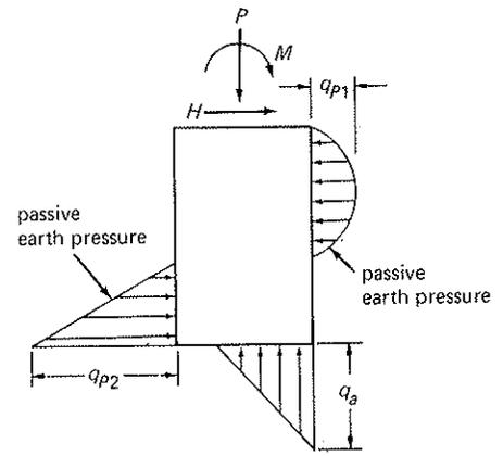
Fig. 5-7 General distribution of base and side pressures of a footing resisting overturning moments, where  $q_{p1}$  and  $q_{p2}$  are passive earth pressures due to loading and  $q_{p1}$  and  $q_{p2}$  are to be  $\leq$  the maximum allowable passive earth pressure that can be utilized at each depth.
