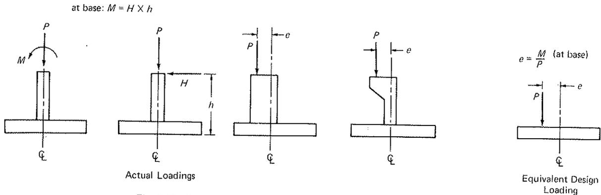
Fig. 5-10 Analogy between moments and eccentric loading conditions.
