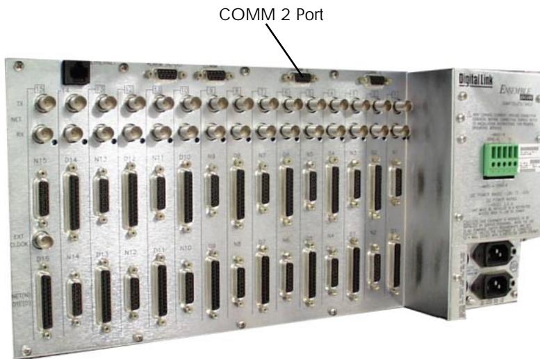
Figure 3-2 COMM2 Connector on Ensemble Shelf
