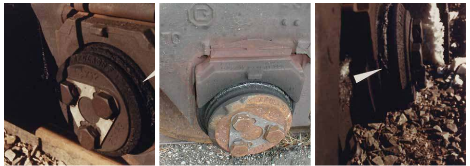
Fig. 4. Old Grease Accumulations (Dried and Covered with Road Dirt).
