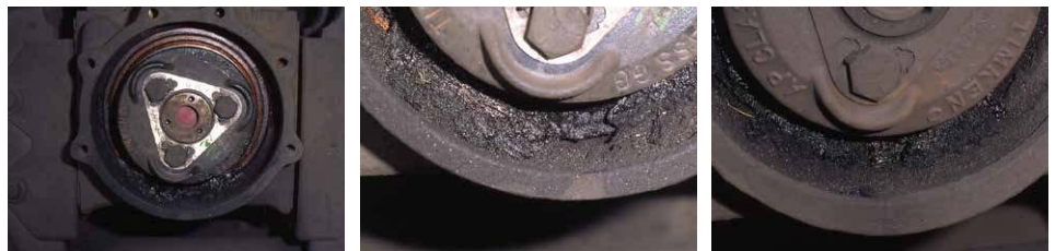
Fig. 3a. Examples of Fresh Grease Leakage (Note Shiny/Wet Appearance Grease).
