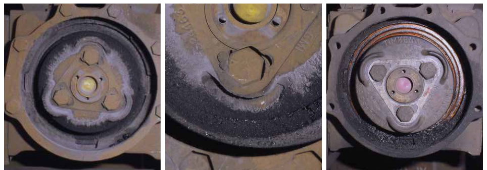
Fig. 4a. Examples of Old Grease Accumulations (Dried and Covered with Road Dirt).
