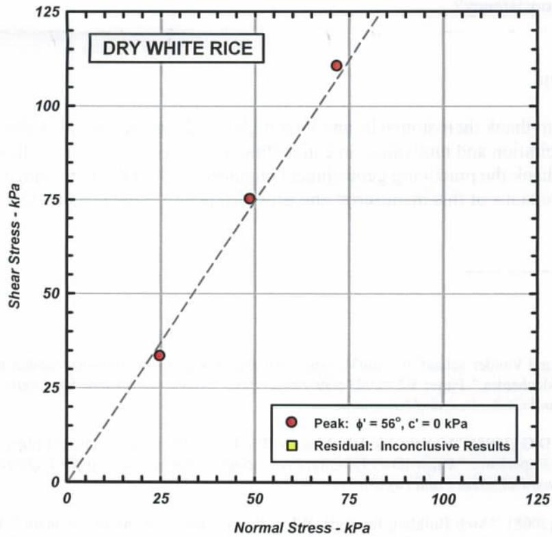
Figure 12 - Direct Shear Test Results for Dry White Rice
