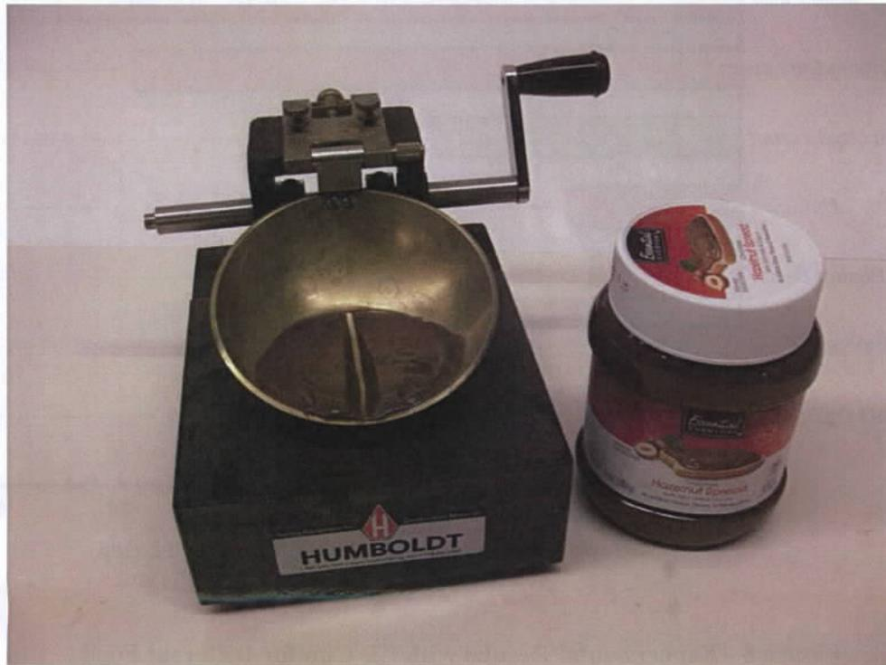
**Figure 7 - Liquid Limit Cup Test on Hazelnut Spread**
