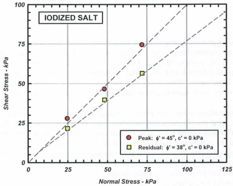
Figure 11 - Direct Shear Test Results for Iodized Salt
