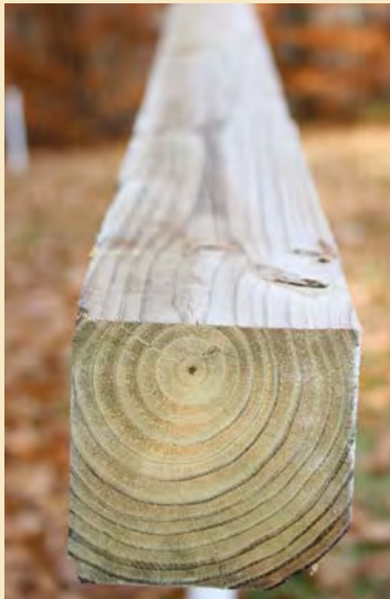
Figure 4. Solid lumber such as a 4x4 or a 4x6 can no longer be used as a beam. Most beams must be built up from layers of 2-by material.
