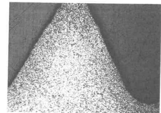
Structure of Case & Core After Anneal at 1600°F (870°C) for 7 minutes — Magnification of 100X, Nital Etch.
