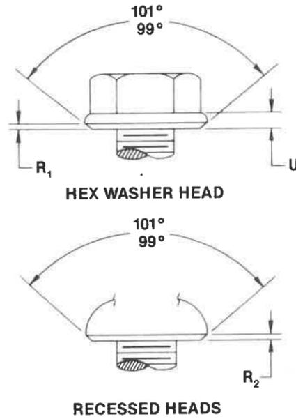
Table 1 Head Chamfer Dimensions for Milled Point Self-Drilling Tapping Screws
