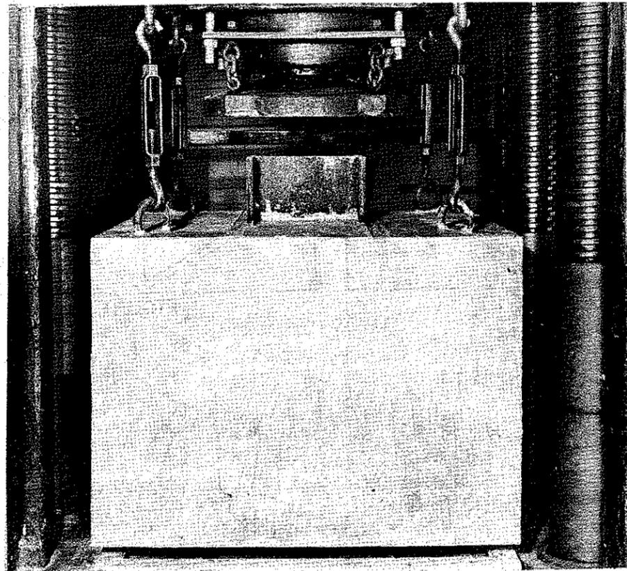
PLATE 2. SERIES C SPECIMEN SUSPENDED ON TURNBUCKLES PEREPARATORY TO ALIGNMENT AND CAPPING.
