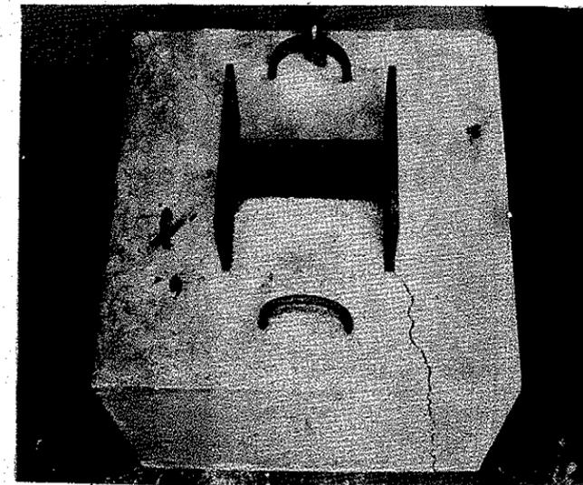
PLATE 5. FAILURE IN CONCRETE BLOCK ON SPECIMEN A-6 WITH 10" X 10" H-PILE.
