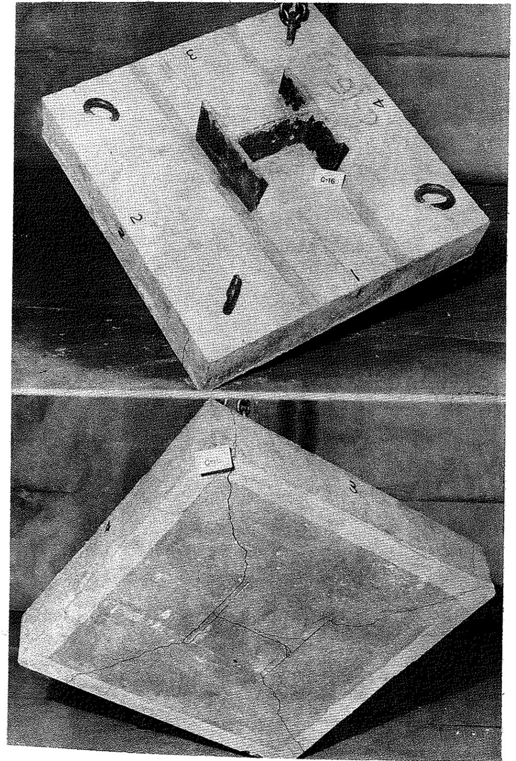
PLATE 25. APPEARANCE OF SPECIMEN C-16 AFTER TESTING.
