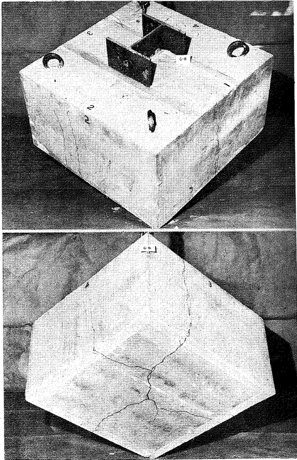
PLATE 18. APPEARANCE OF SPECIMEN C-8 AFTER TESTING.
