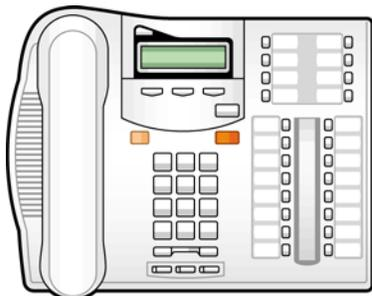
The T7316E telephone is part of the BST portfolio. It has 24 fully programmable buttons. 16 of the programmable buttons are supported by LCD indicators (for one button access to a combination of lines, features and autodial numbers). Release 6.1 software is required to program lines for all 16 buttons. Earlier versions of software allow up to ten lines to be programmed for line appearances.
