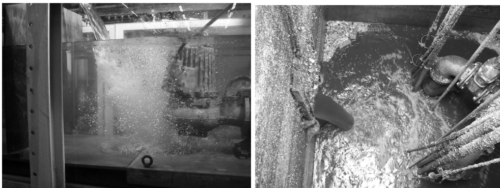
Figure 2.1 Air entraining plunging jets in the lab (Kranendonk, 2007) and the field
