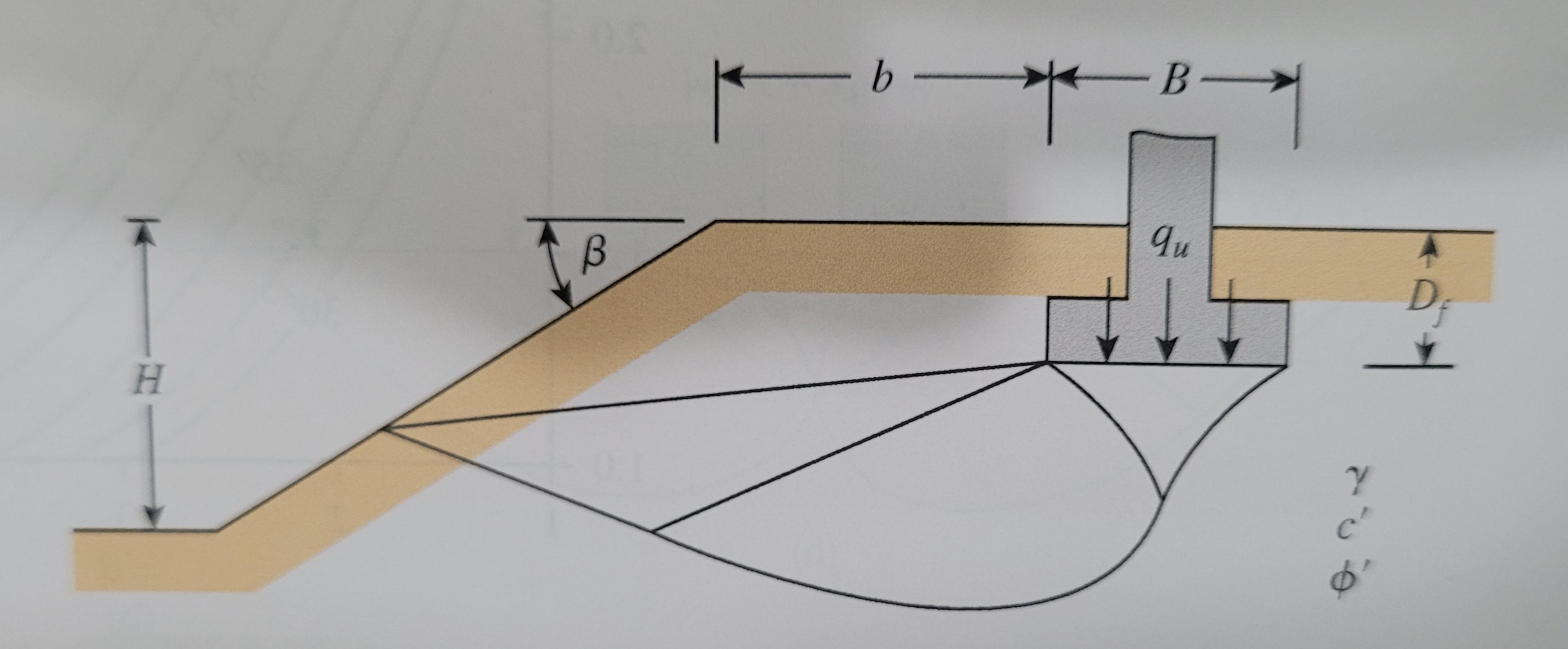
FIGURE 7.19 Shallow foundation on top of a slope
