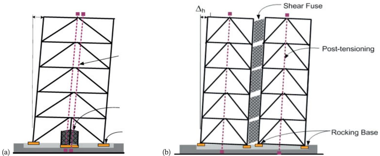
Fig. 2. Controlled rocking frame configurations; (a) single frame, (b) dual Frames
