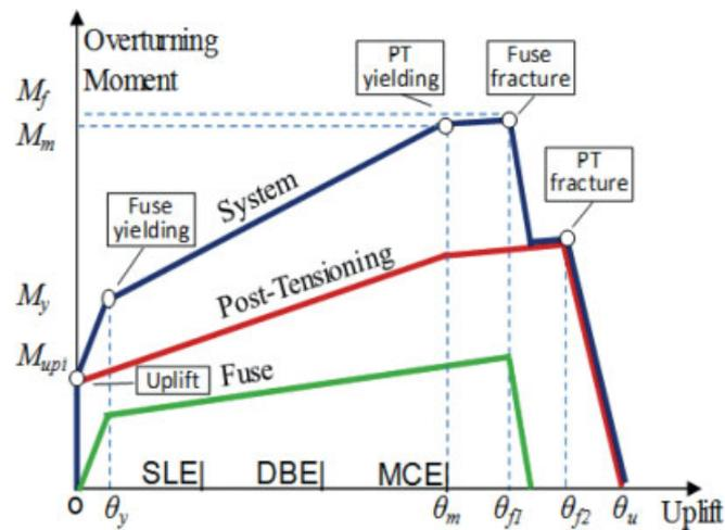
Fig. 7. Idealized static nonlinear response with critical limit states
