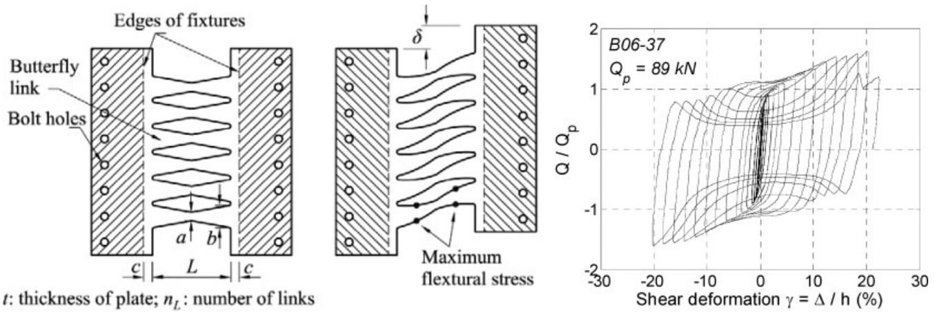
Fig. 3. Energy dissipating steel butterfly-shaped fuses
