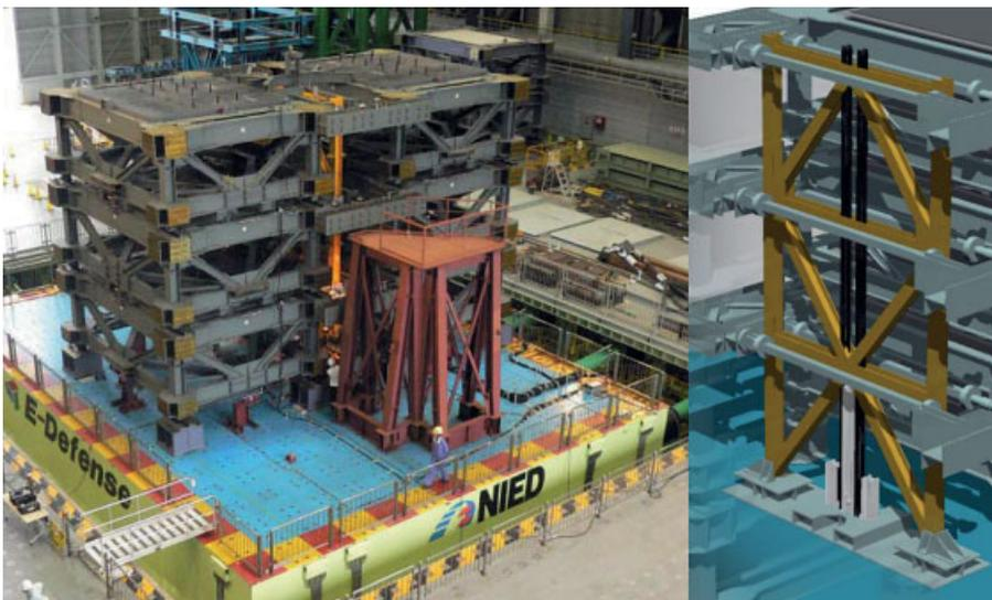
Fig. 5. E-Defense shaking table test of three-story frame specimen with seismic mass testbed simulator
