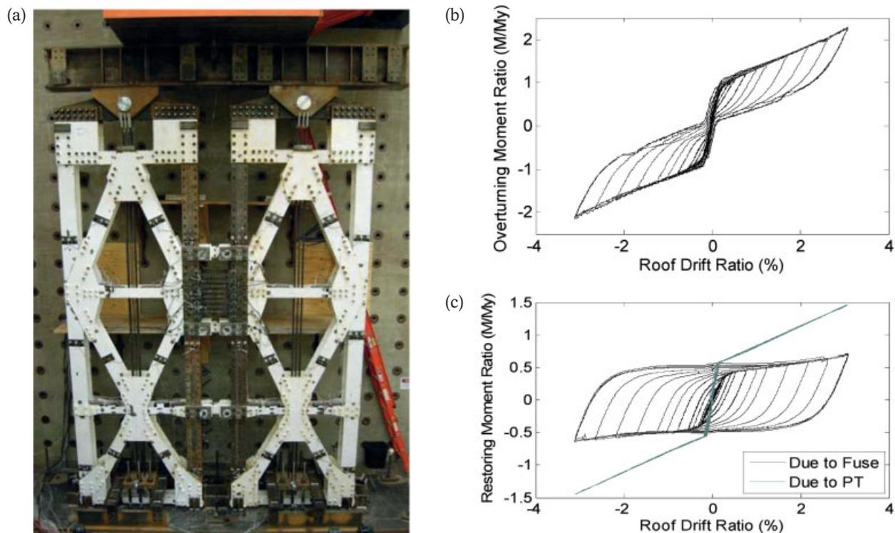
Fig. 4. Quasi-static cyclic testing of dual frame specimens; (a) test specimen, (b) overall hysteretic response, (c) components of hysteretic response
