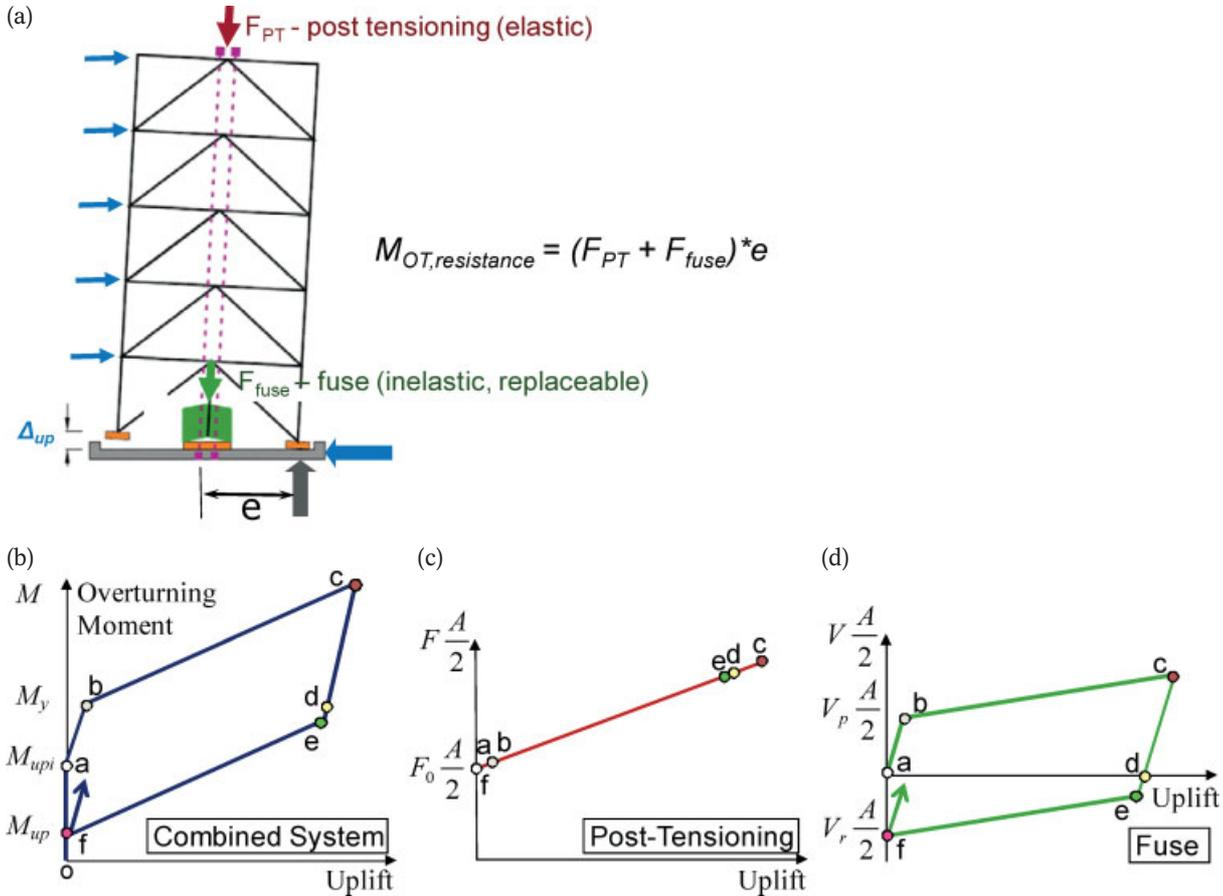
Fig. 1. Rocking frame; (a) schematic free-body diagram, (b) combined system response, (c) steel post-tensioning response, and (d) energy dissipating fuse response
