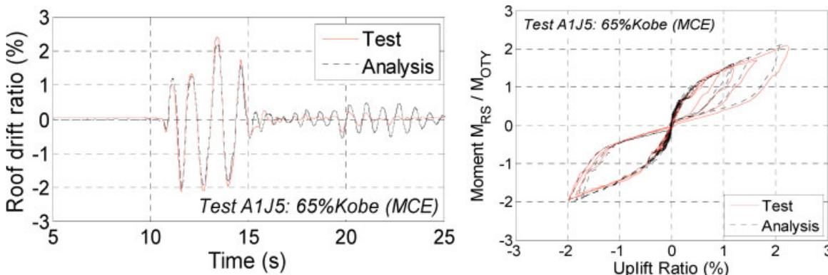
Fig. 6. Shaking table results: JMA Kobe motion scale to MCE intensity
