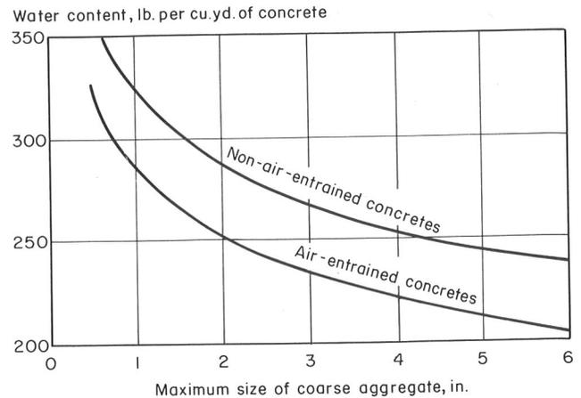
Fig. 15. The water requirement for concrete of a given consistency decreases as the maximum size of coarse aggregate increases.
