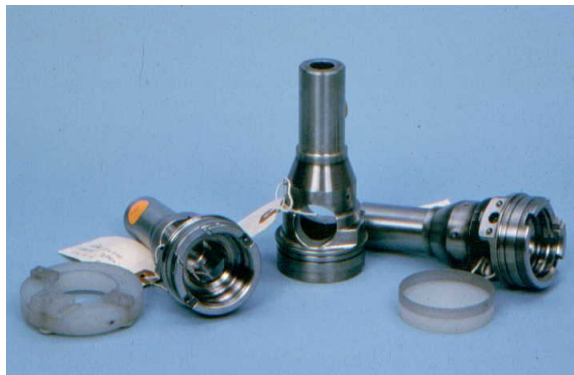
Figure 6.2: Wing pivot shaft masking fixture.
