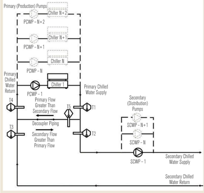
FIGURE 2 Decoupler piping.
