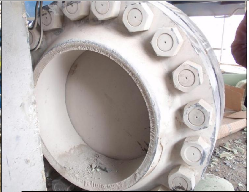
Apparent failed 36" flange
