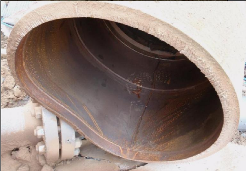
Apparent failed 36" flange
