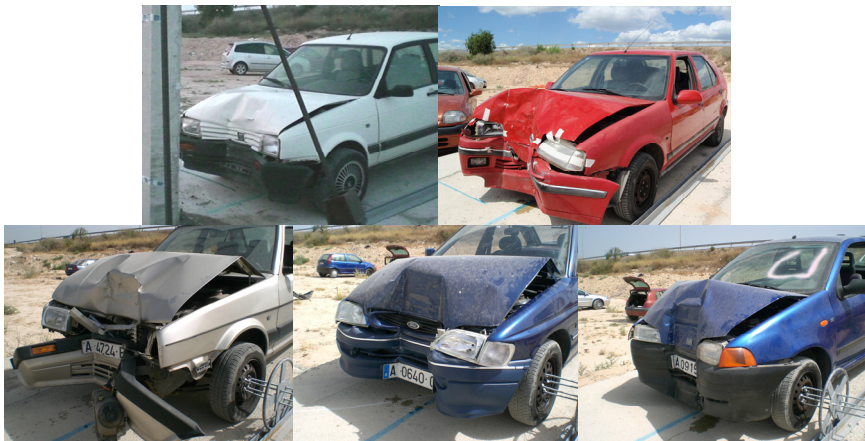
Figure 6: Final car condition after the experiments: Seat Ibiza, Renault 19 Chamade, Seat Málaga, Ford Escort, Fiat Punto.
