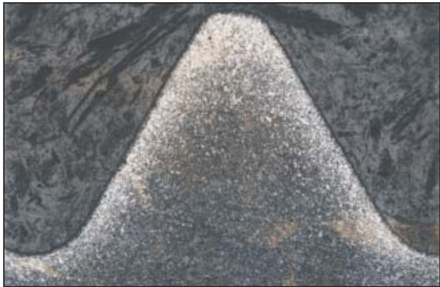
Figure 1 Definition of Partial Decarburization Limits (federal Specification, FF-S-86, screw, cap, socket head)
