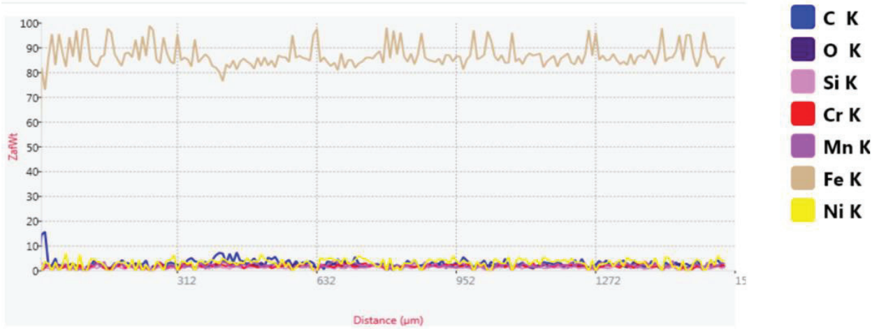
Fig. 5 The line scan results from Figure 4 are presented. No significant change in relative surface composition was observed.
