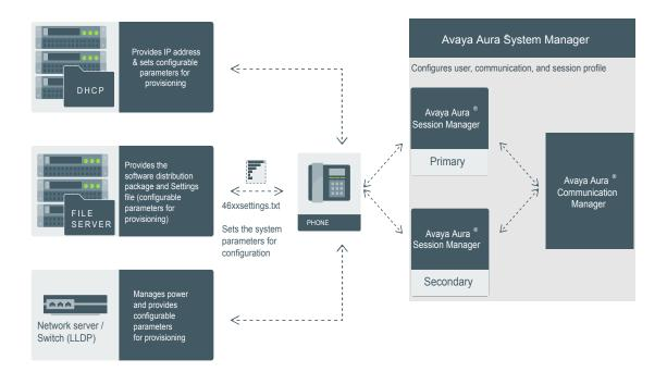
Figure 1: Diagram: Phone setup in Avaya Aura® environment
