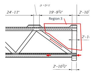
d. There appears to be significant shear lag issues in both the canopy and walkway as the stiff web element is being dragged behind the compression zone. The designer needs to pay particular attention in these areas. Moving the canopy continuity tendon to the middle tendon spot may improve the issue. Consider adding addional longitudinal tendons in the added 2 ft. corner chamfers (Comment 4.c.i).
