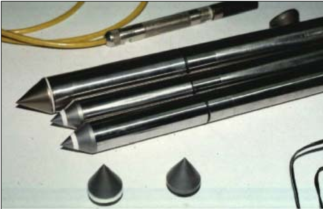
Figure 5.1b Cone Penetrometers (from Mayne et. al., 2002)
