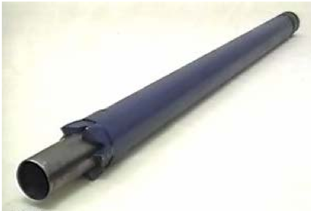
Figure 4.8. Pitcher Sampler from Mayne, et. al., (2002)
