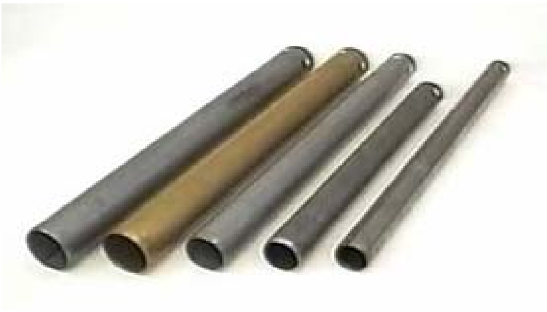
Figure 4.7b Various Diameter Shelby Tubes from Mayne, et. al., (2002)
