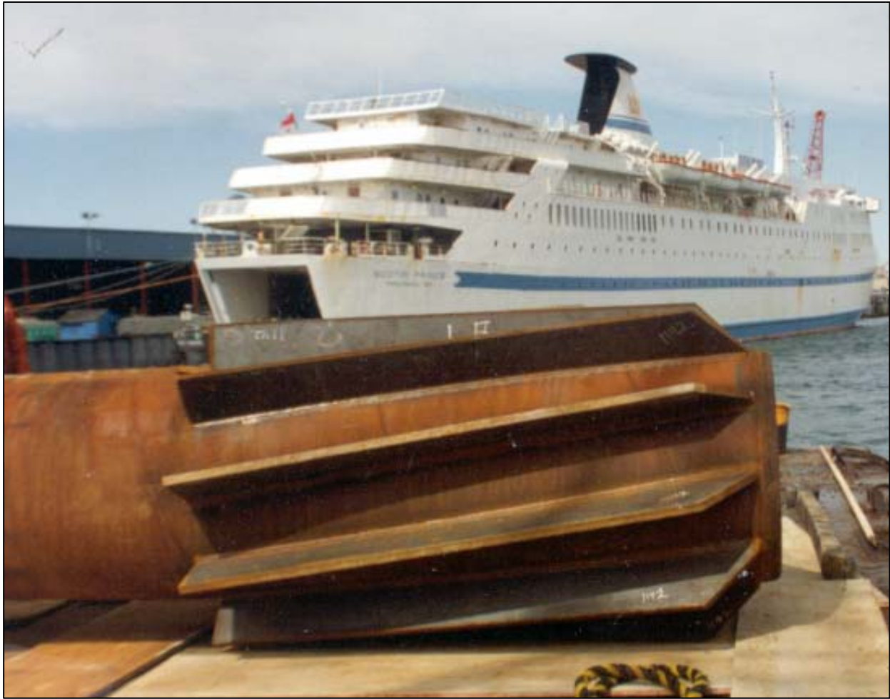
Figure 8.6 760 mm (30 inch) Diameter Spin Fin Pile
