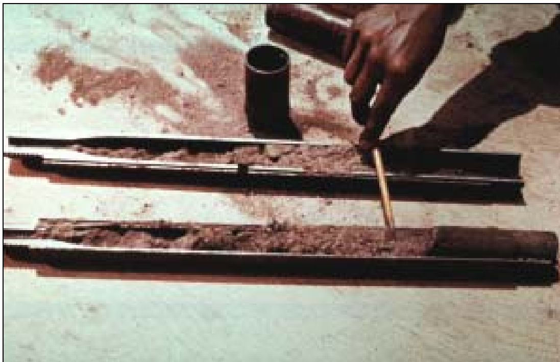
Figure 4.3 Split Barrel Sampler from Mayne et. al., (2002)
