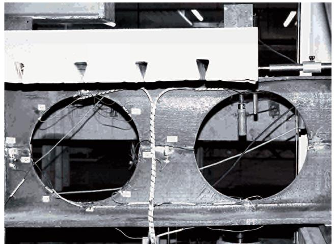
**Figure 2-26: Vierendeel mechanism - Test 3**
