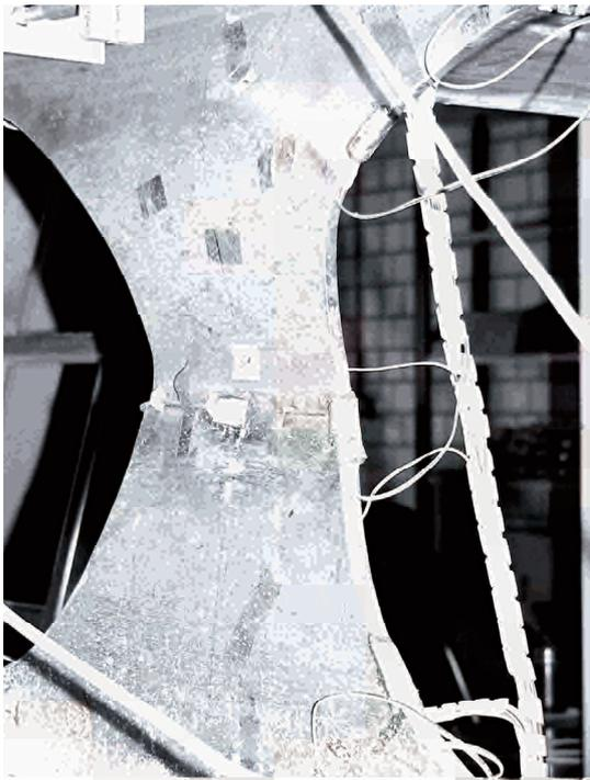
**Figure 2-25: Web post buckling - Test 3**
