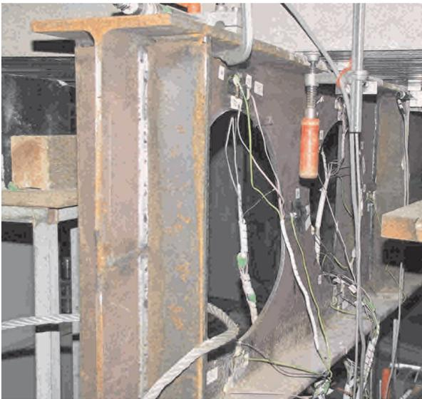
**Figure 2-16: Flexural web post buckling between opening 11 and 12 - Test 1A**
