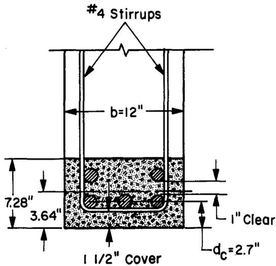
**Fig. 10-2 – Effective tension area of concrete (beam with five #11 bars)**
