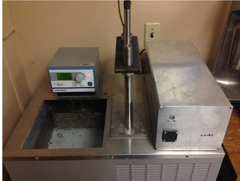
Figure A.1 Thermal Bath used for AASHTO T336.
