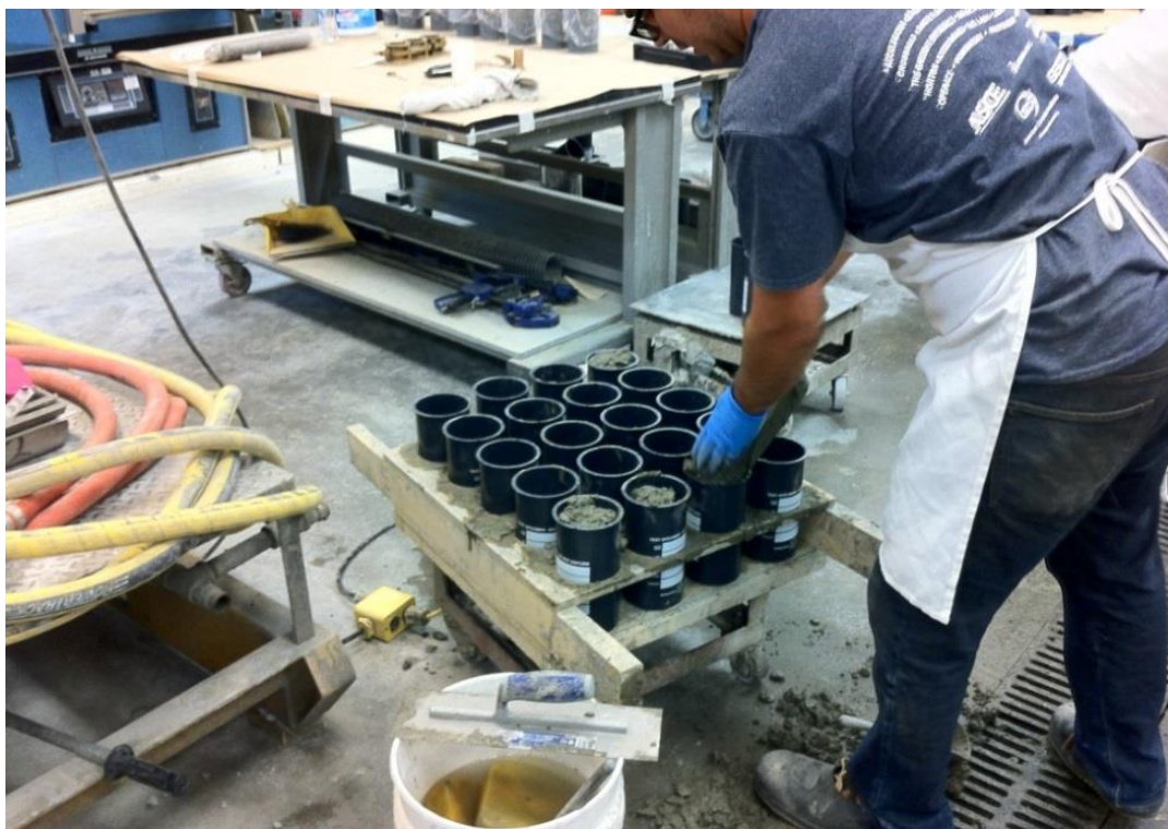
Figure 6.7 Placement of concrete in cast specimens
