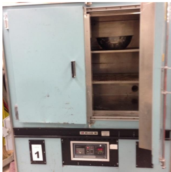
Figure 6.2 Moisture coarse aggregate sample placed in oven
