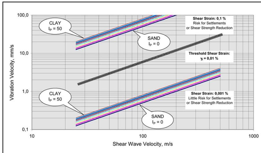
Figure 6 - Estimation of risk for settlement or strength reduction from vibration velocity as a function of shear wave velocity for different levels of shear strain
