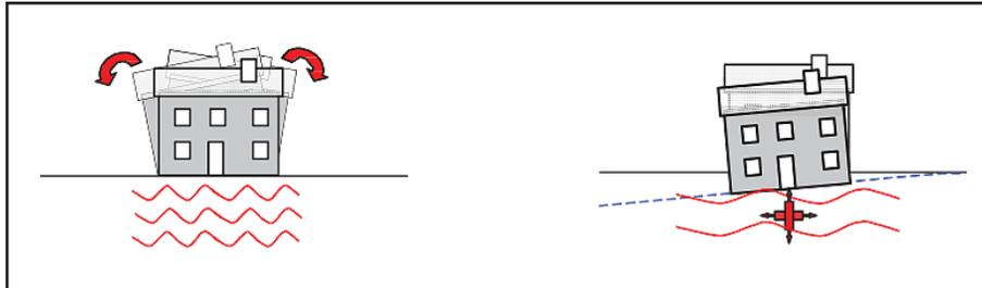
Figure 3 – A building’s reaction to direct dynamic effects (on left) and indirect settlement (on right)
