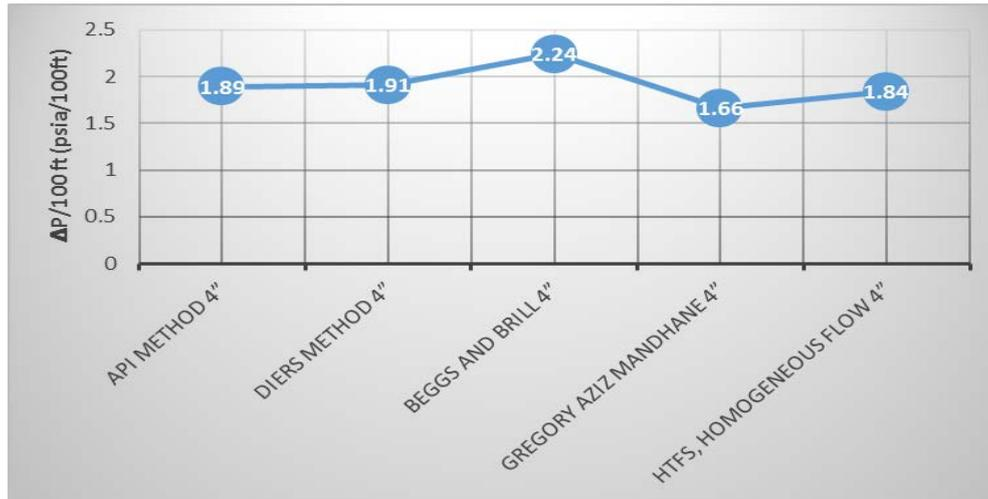
**Figure 2.** Comparison between different 2-phase flow models.
