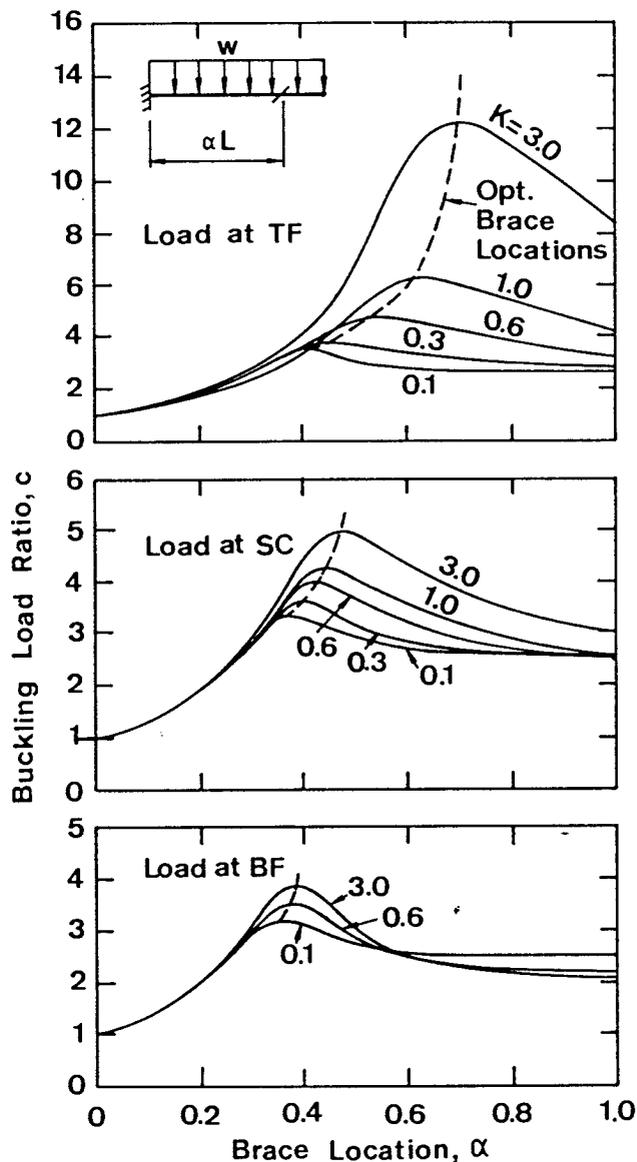
Fig. 32 — Buckling Load Ratios for Cantilevers with Uniformly Distributed Load and a Full Brace.
