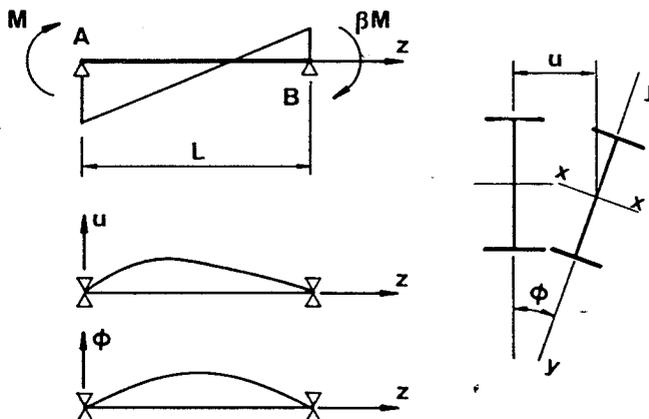
Fig. 4 — Simply Supported Beam with End Moments.
