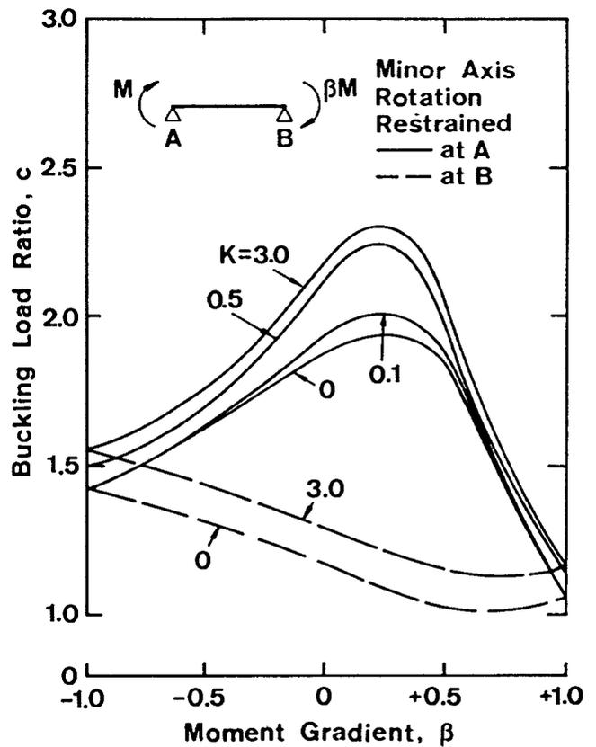
Fig. 7 — Buckling Load Ratios for Moment Gradient Beams with One End Restrained Against Minor Axis Rotation.
