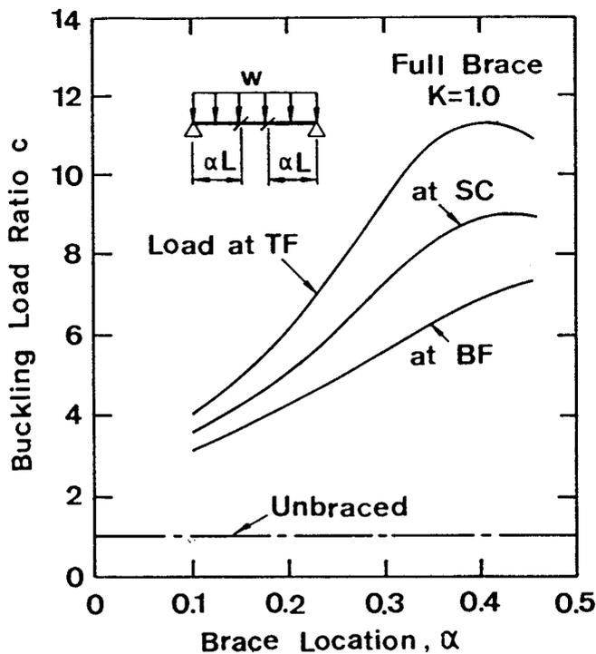
Fig. 28 — Influence of Load Height on Simply Supported Beams with Uniformly Distributed Load and Two Full Braces.
