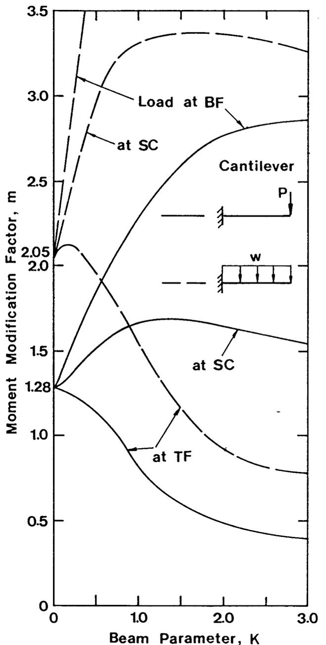
Fig. 21 — Moment Modification Factors for Cantilevers.
