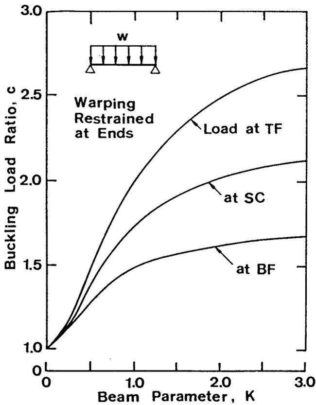
Fig. 17 — Buckling Load Ratios for Warping End Restrained Beams with Uniformly Distributed Load.
