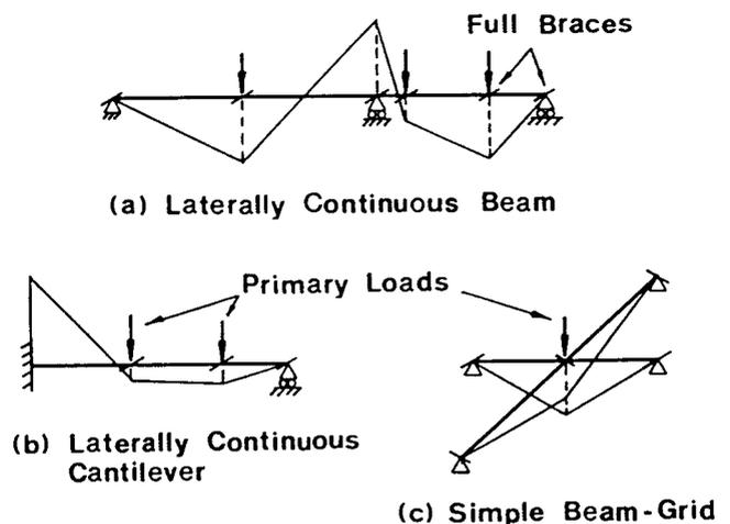
Fig. 37 — Laterally Continuous Structures.
