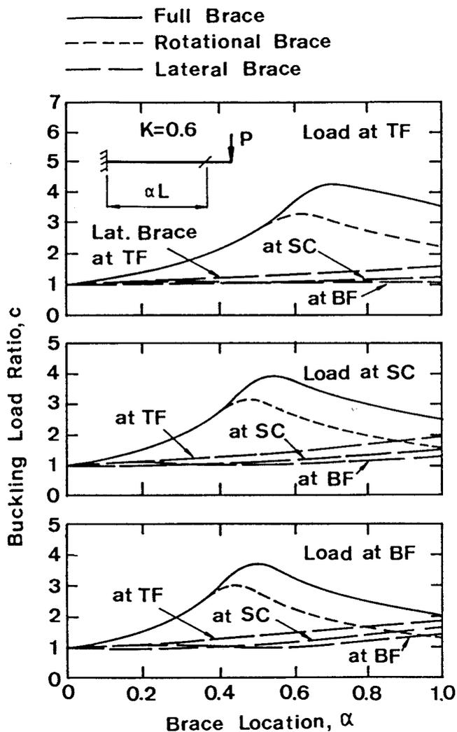
Fig. 33 — Comparison of Brace Types for Cantilevers with a Tip Load,  $K = 0.6$ .
