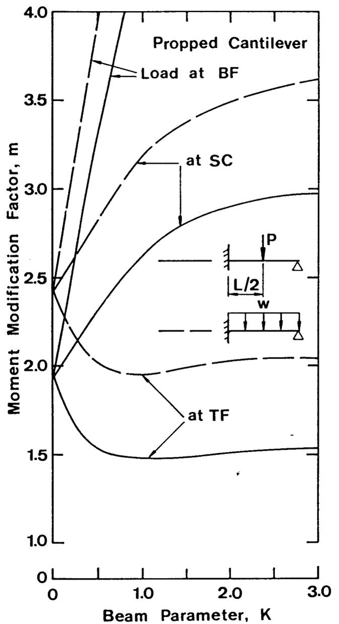
Fig. 19 — Moment Modification Factors for Propped Cantilevers.
