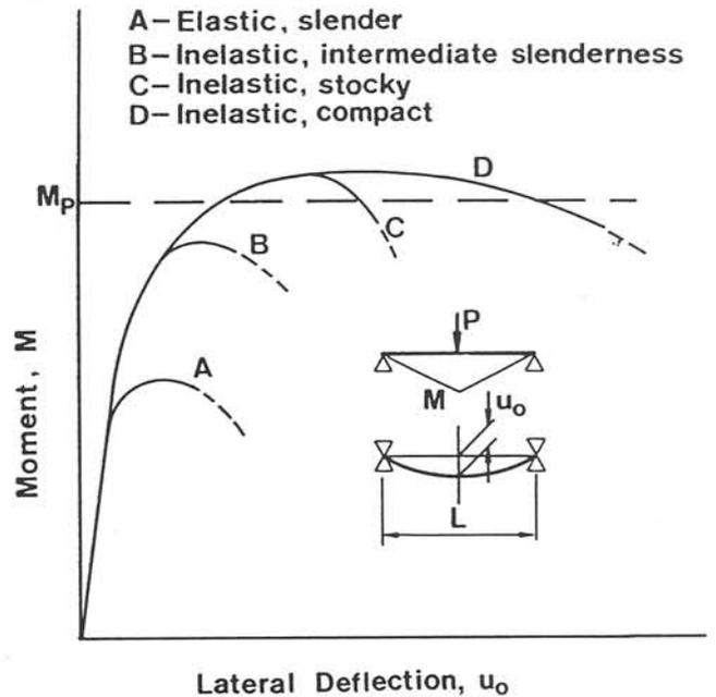
Fig. 2 — Load-Deformation Behaviour of Typical I-Beam.
