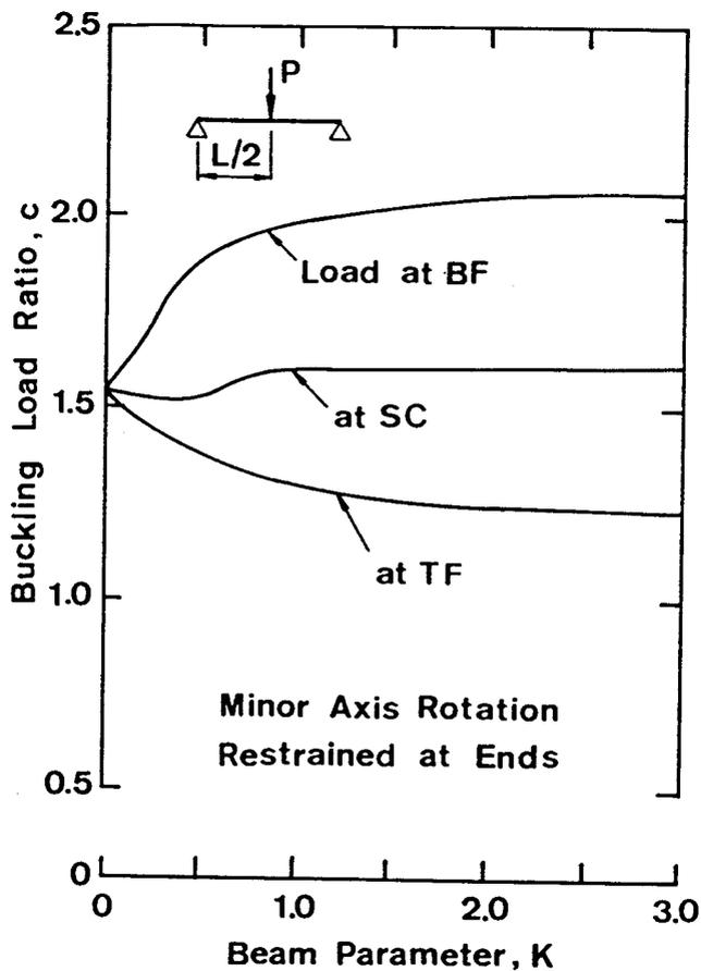
Fig. 14 — Buckling Load Ratios for Minor Axis Rotation End Restrained Beams with Central Point Load.
