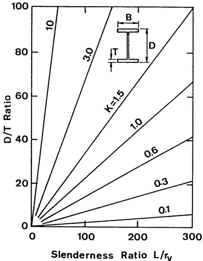
Fig. 5 — Variation of Beam Parameter,  $K$ .
