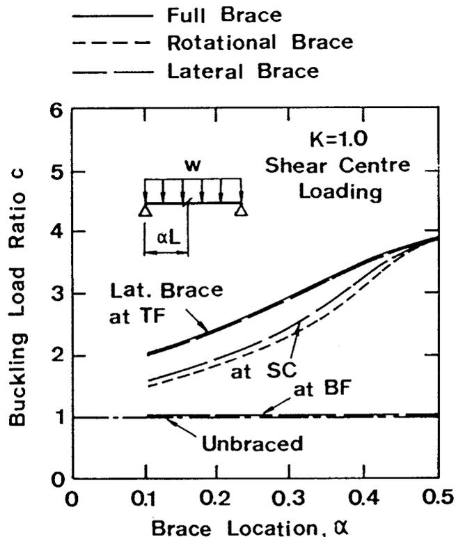
Fig. 29 — Comparison of Brace Types for Simply Supported Beams with Uniformly Distributed Load,  $K = 1.0$ .
