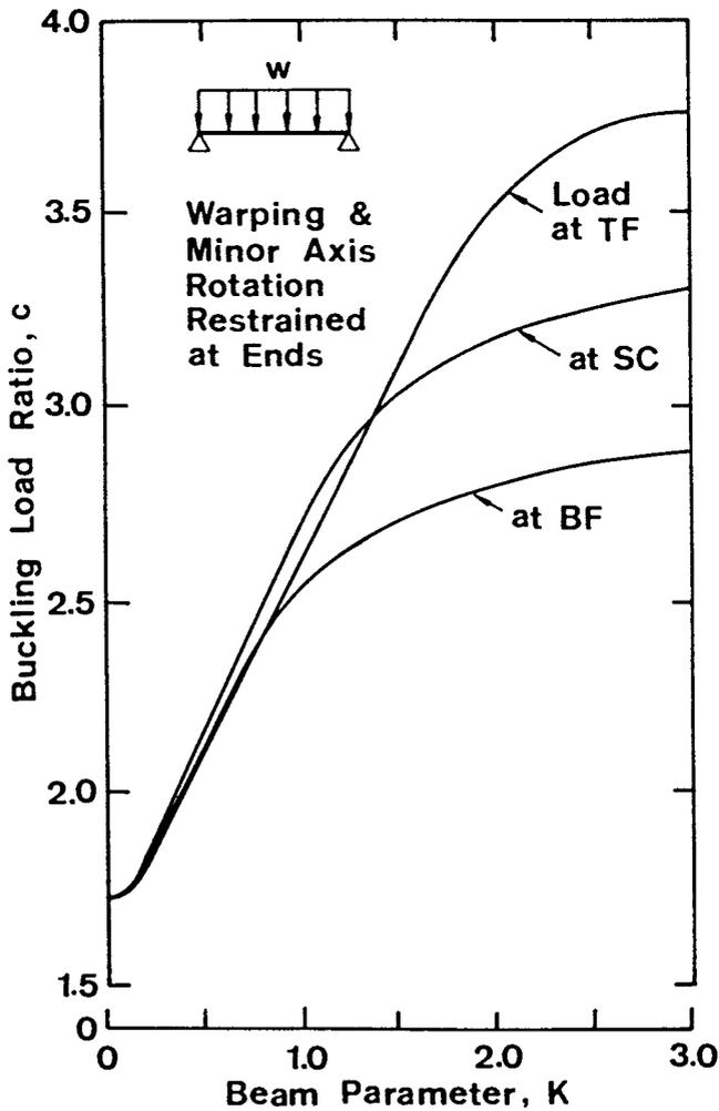
Fig. 18 — Buckling Load Ratios for Warping and Minor Axis Rotation End Restrained Beams with Uniformly Distributed Load.
