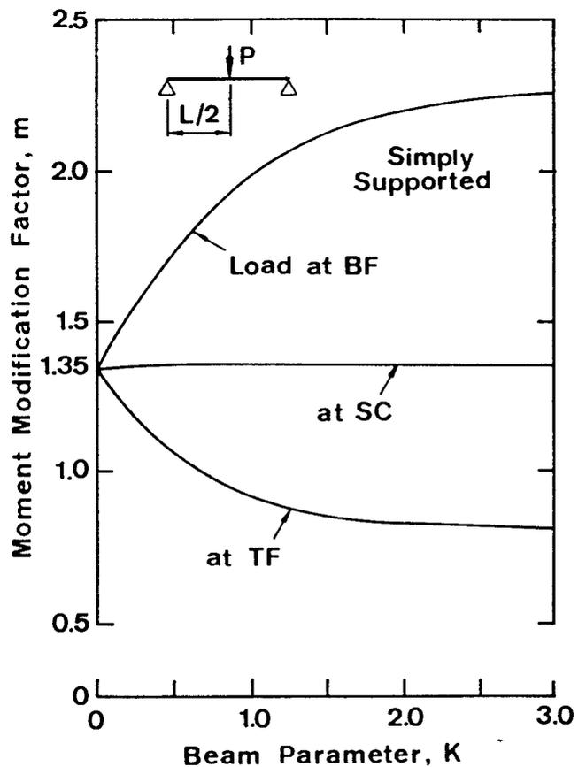
Fig. 12 — Moment Modification Factors for Simply Supported Beams with Central Point Load.
