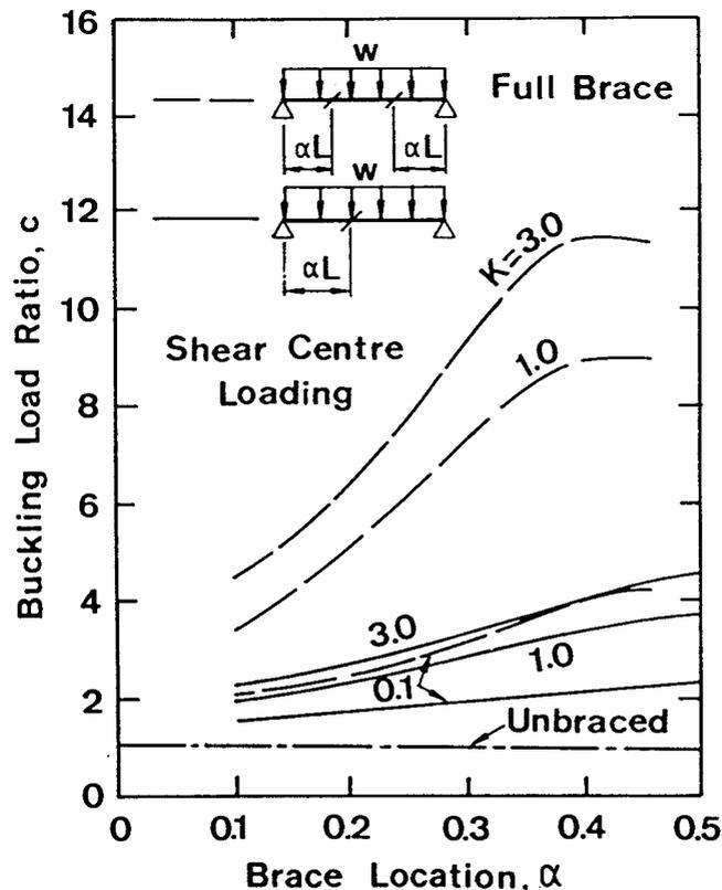
Fig. 27 — Buckling Load Ratios for Simply Supported Beams with Uniformly Distributed Load and One or Two Full Braces.
