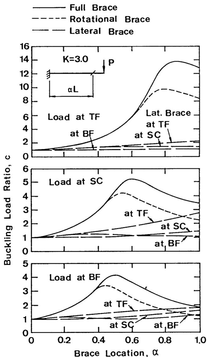
Fig. 34 — Comparison of Brace Types for Cantilevers with a Tip Load,  $K = 3.0$ .
