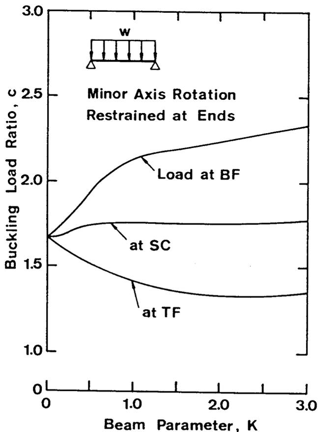
Fig. 15 — Buckling Load Ratios for Minor Axis Rotation End Restrained Beams with Uniformly Distributed Load.
