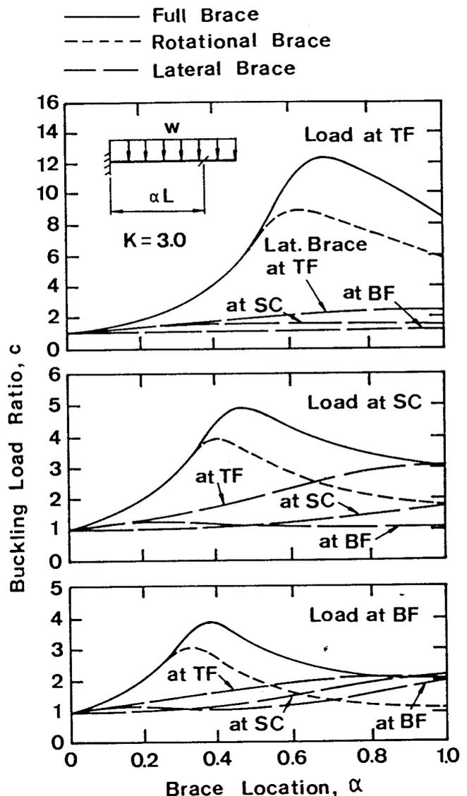
Fig. 36 — Comparison of Brace Types for Cantilevers with Uniformly Distributed Load,  $K = 3.0$ .
