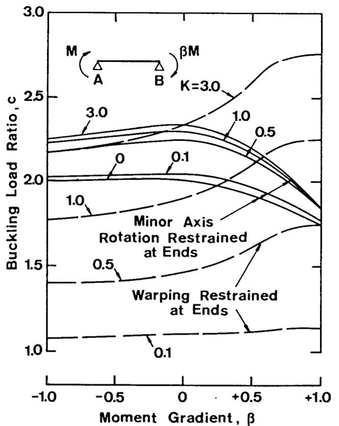
Fig. 8 — Buckling Load Ratios for Moment Gradient Beams with Both Ends Restrained against Minor Axis Rotation or Warping.
