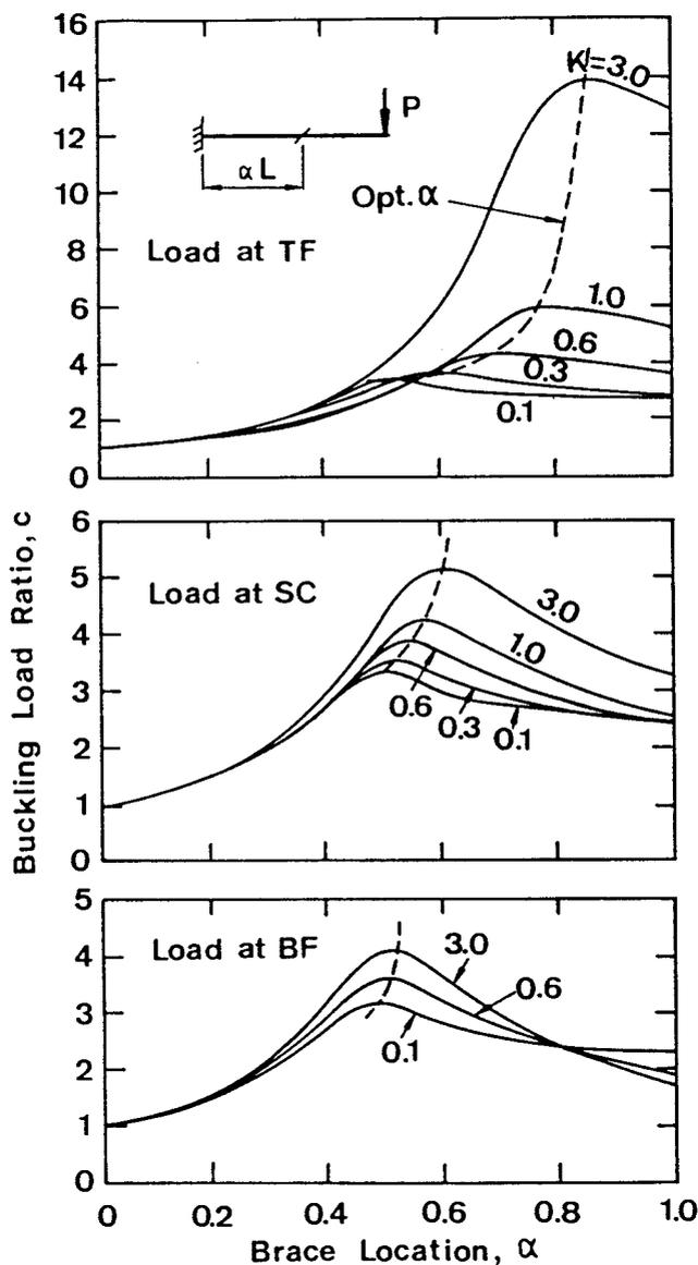
Fig. 31 — Buckling Load Ratios for Cantilevers with a Tip Load and a Full Brace.
