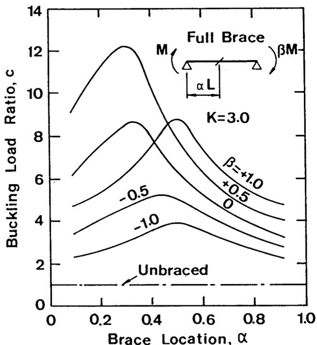
Fig. 26 — Buckling Load Ratios for Simply Supported Beams with End Moments and a Full Brace,  $K = 3.0$ .
