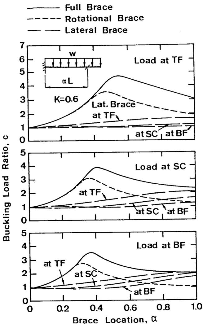
Fig. 35 — Comparison of Brace Types for Cantilevers with Uniformly Distributed Load,  $K = 0.6$ .
