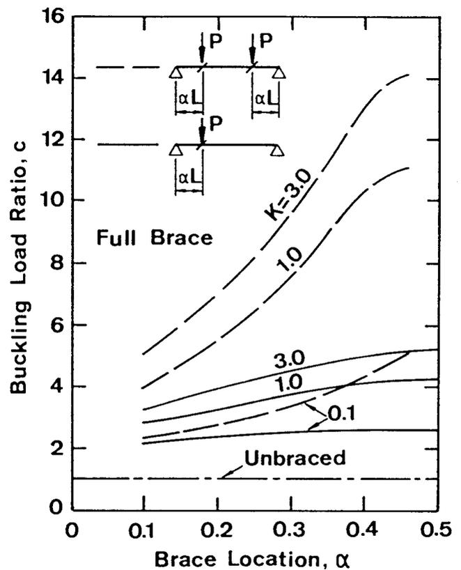
Fig. 24 — Buckling Load Ratios for Simply Supported Beams with One or Two Point Loads and Full Braces.
