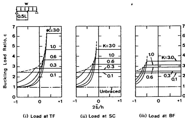
Fig. 30 — Influence of Lateral Brace and Load Height for Simply Supported Beams.
