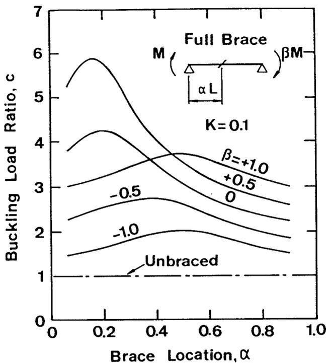
Fig. 25 — Buckling Load Ratios for Simply Supported Beams with End Moments and a Full Brace,  $K = 0.1$ .
