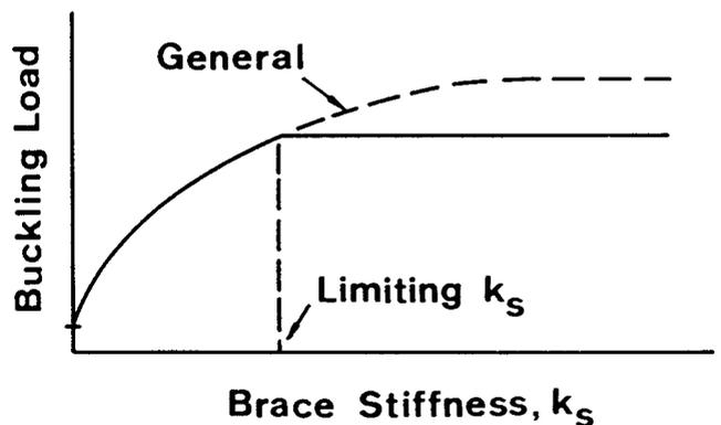
Fig. 22 — Typical Relationship Between Buckling Load and Brace Stiffness.
