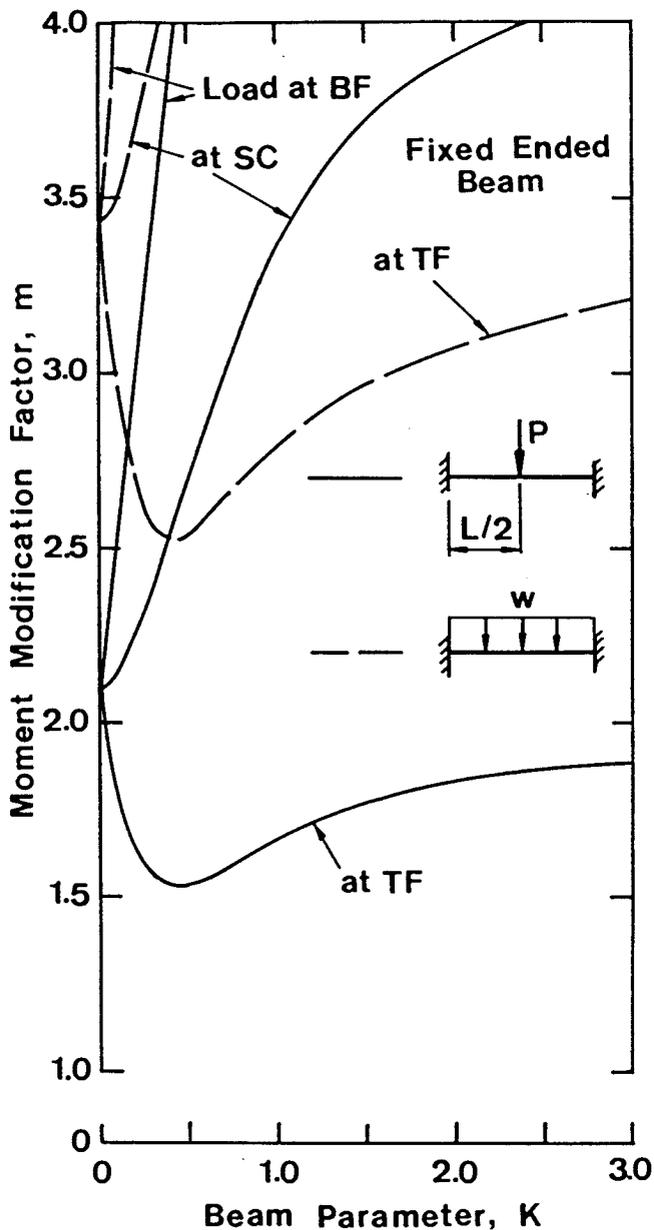
Fig. 20 — Moment Modification Factors for Fixed Ended Beams.
