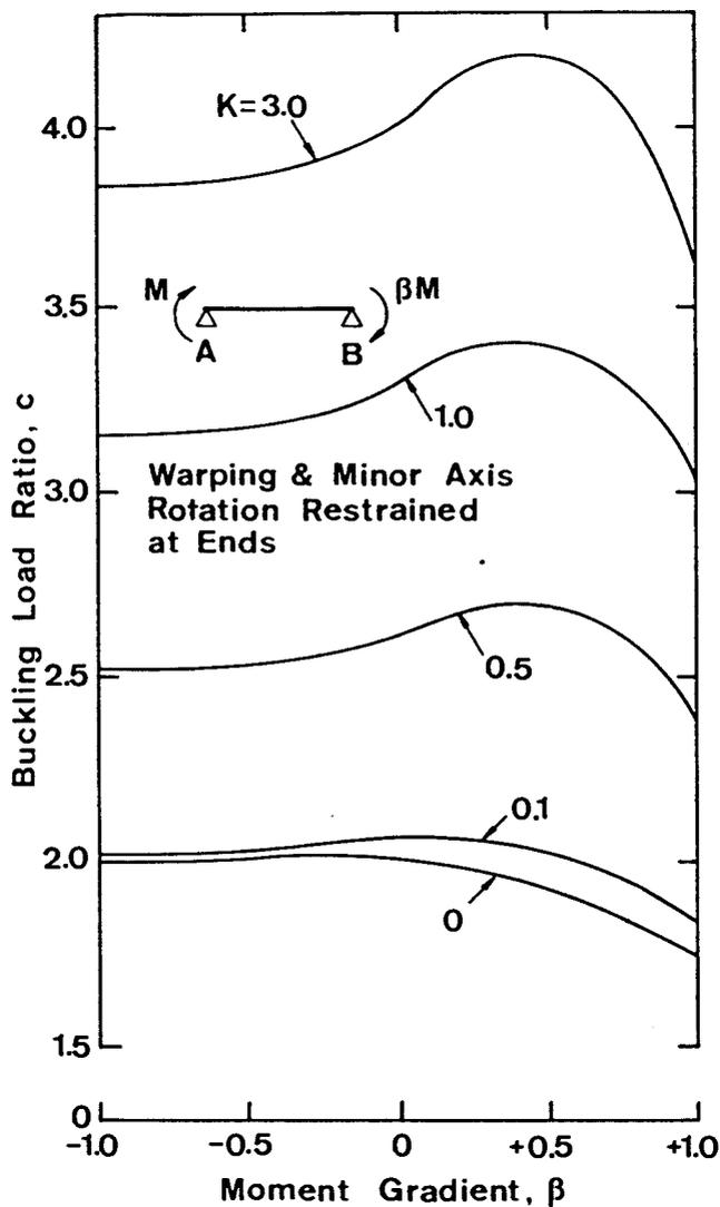
Fig. 11 — Buckling Load Ratios for Moment Gradient Beams with Both Ends Restrained Against Warping and Minor Axis Rotation.
