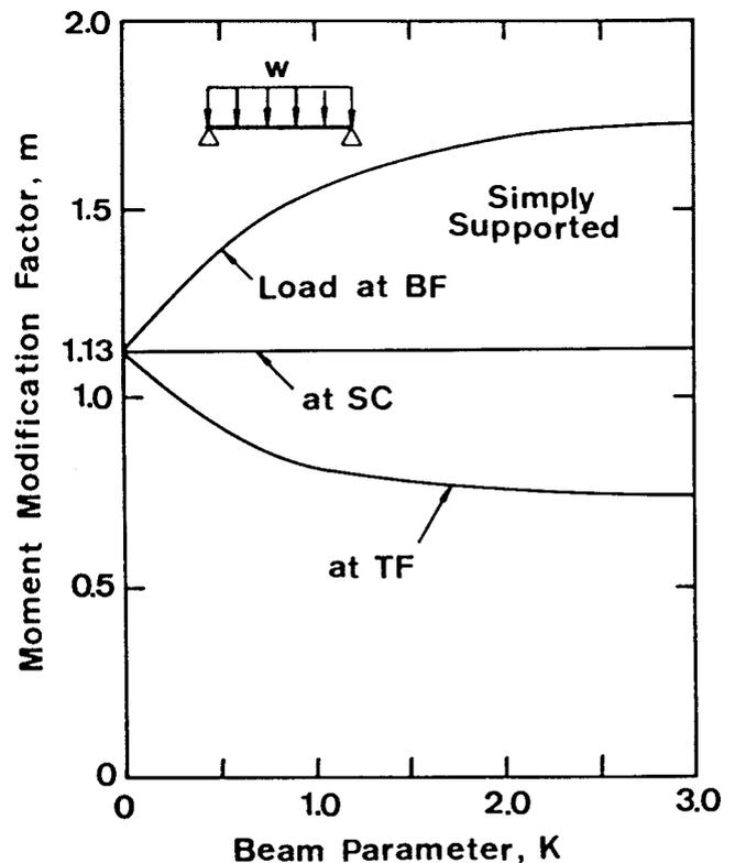
Fig. 13 — Moment Modification Factors for Simply Supported Beams with Uniformly Distributed Load.
