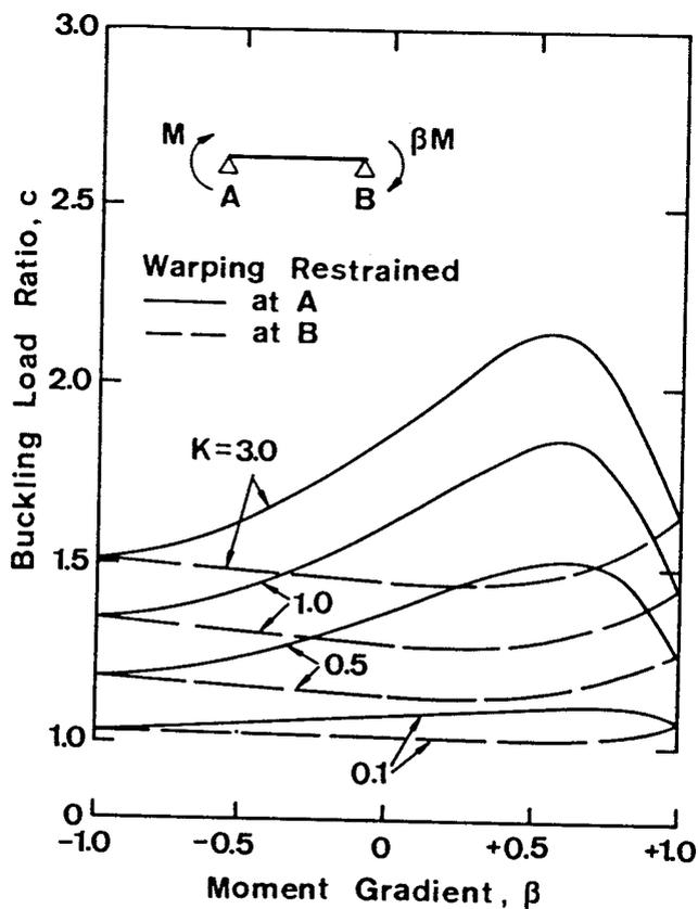
Fig. 9 — Buckling Load Ratios for Moment Gradient Beams with One End Restrained Against Warping.
