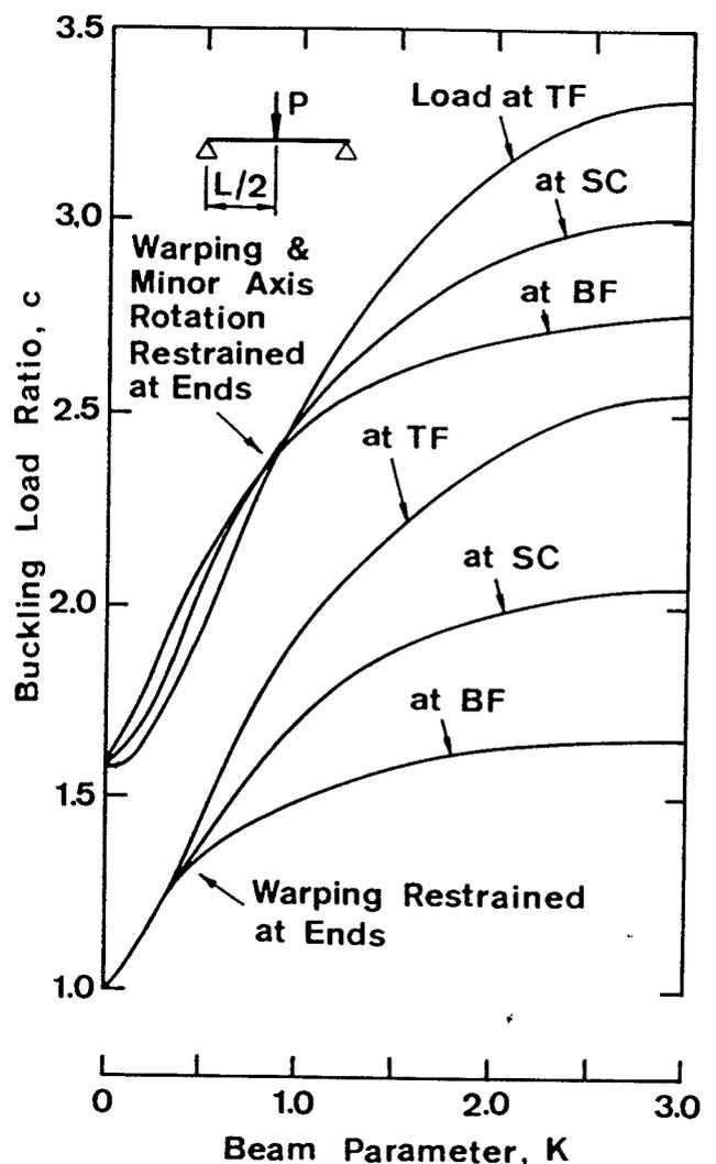
Fig. 16 — Buckling Load Ratios for Warping and Minor Axis Rotation End Restrained Beams with Central Point Load.
