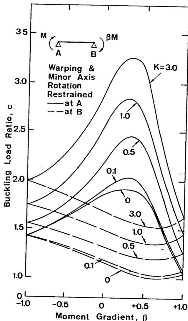
Fig. 10 — Buckling Load Ratios for Moment Gradient Beams with One End Restrained Against Warping and Minor Axis Rotation.
