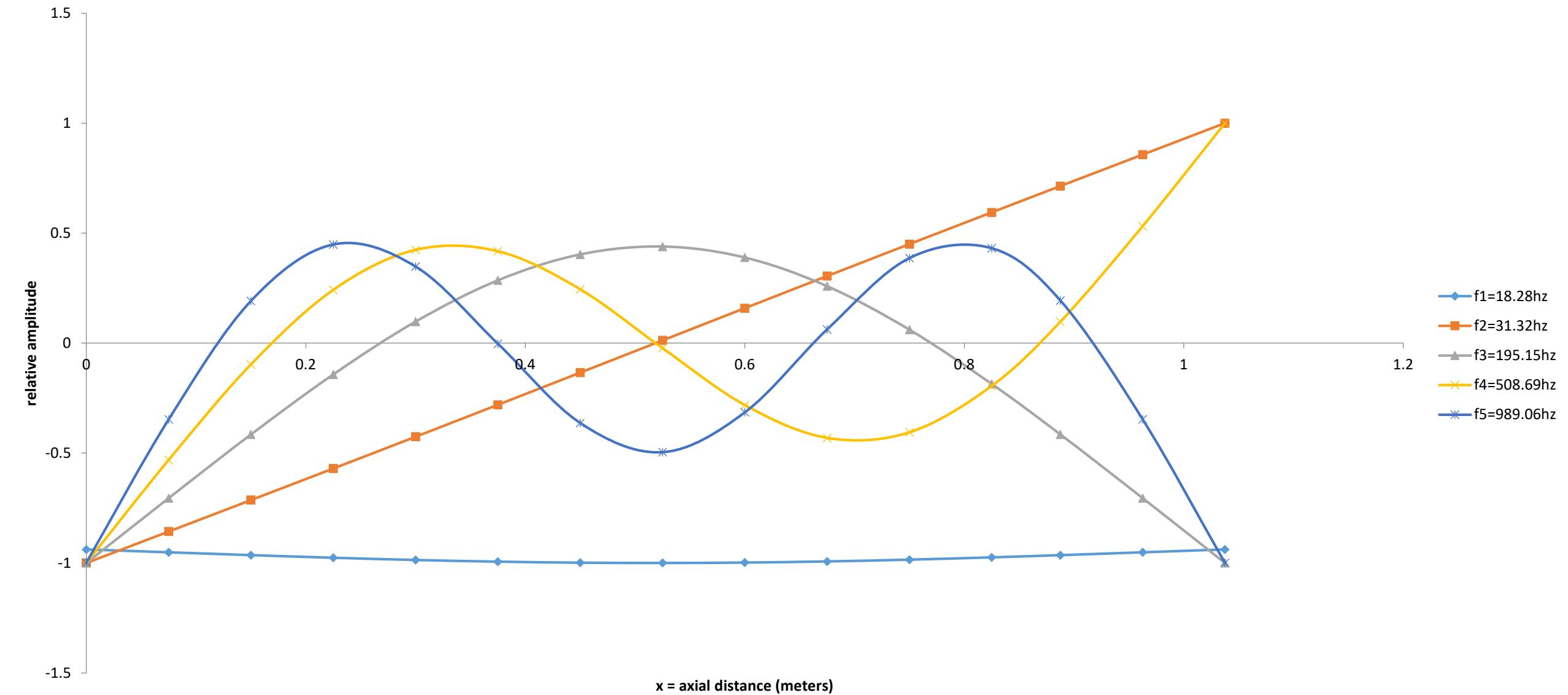
Bearing stiffness multiplier of 1. First resonant frequency is flexible rotor modeshape, however it is at 84hz.
