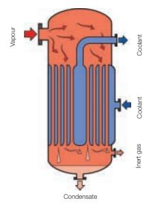
Working closely with our customers helps them to optimize their processes and introduce new forms of heat exchange – such as this fully built condensing tower with three spiral bodies.
