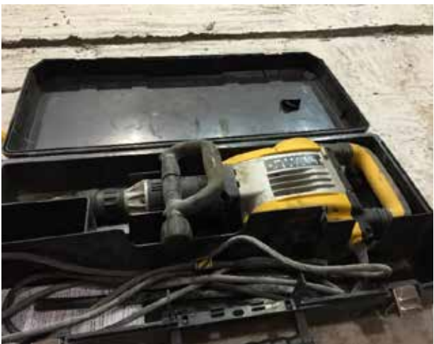
(c) Variable Impact Demolition Hammer
