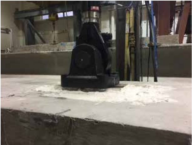
(c) Bearing of Actuator on Bridge Deck
