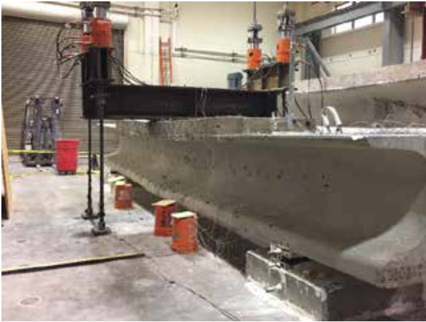
(c) Large Deformation at End of Test
