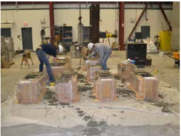
(c) Casting Concrete
