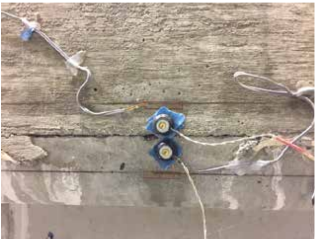
(e) Infrared Markers for Position Tracking
