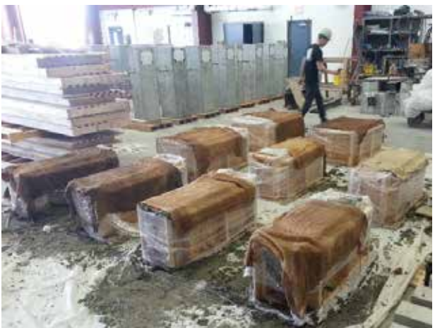
(e) Concrete Curing
