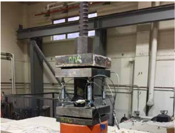
(c) Load Cell Arrangement
