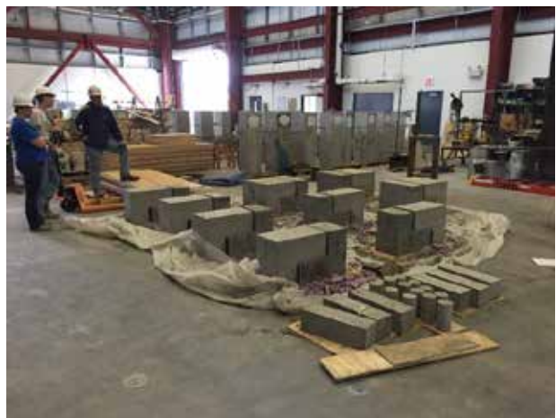
(f) Push-Off Specimens after Demolding
