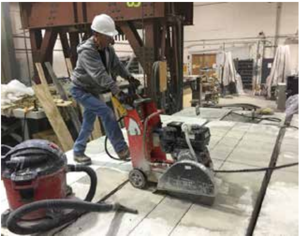
(c) Transverse Saw-Cuts
