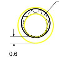
Potential circularity error (in terms of the "two coaxial circles a specified distance apart") as defined by the circularity control
