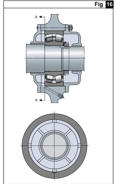
**Figure 16. Roller Bearing Arrangement for Large Electric Motor**
