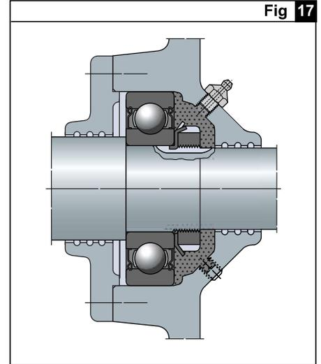
**Figure 17. Grease Chamber for Electric Motor**
